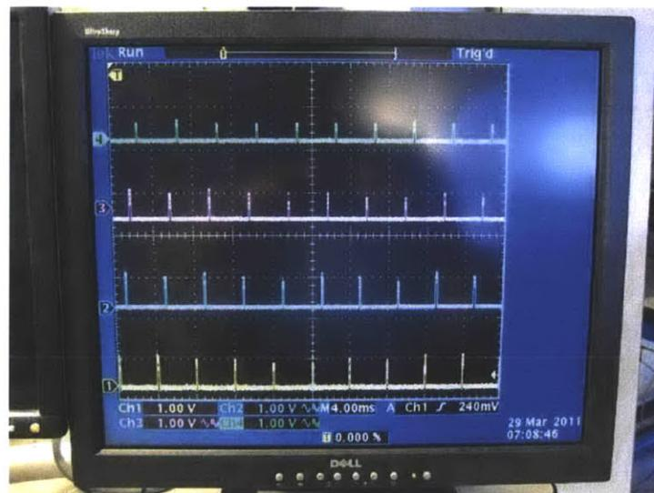
Figure 6.3 – Stimulation pulses from prototype cochlear implant system
