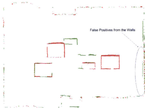
Figure 7-2: Walls should not be considered changes, but as the pose estimates are updated with the additions and removal of constraints some measurement from walls will not coincide. As a result, changes are detected.
