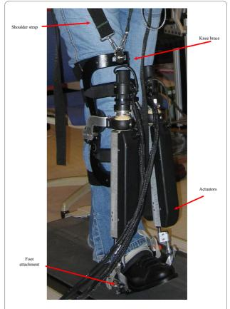
**Figure 1 Anklebot**. The figure identifies the main components of the device.
