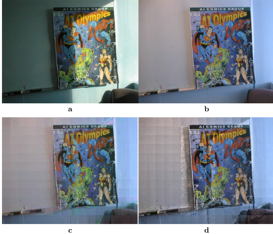
Figure 4: a. Image with strong shadow. b. The same image under more uniform lighting conditions. c. Color flow from a to b using patchwise eigenflows. By clustering flow coefficients, we hope to be able to define the shadow boundary. d. Flow from a to b using the patchwise version of a competitive color mapping model (see [7] for details). Notice the strong artifacts in the competitive color mapping scheme.
