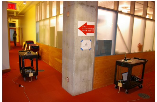
Fig. 2. The measurement setup for collecting waveforms between D675CA and H6 around the corner of the WCNS Laboratory.
