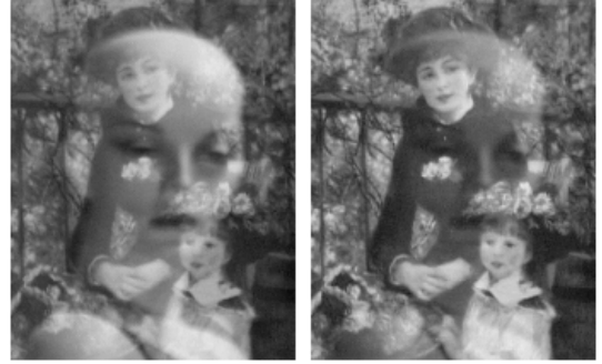
Figure 1: Renoir’s On the Terrace with a reflection of Sheila photographed through a linear polarizer at orthogonal orientations, maximizing and minimizing the reflection.
