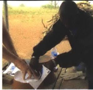
Cutting out a circle of paper to the same size as the filter bottom
