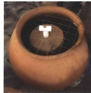
Figure 53 Wire Mesh Restraint System
