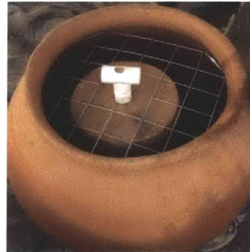
Figure 32 Wire Mesh Restraint System to Submerge and Secure KWK
