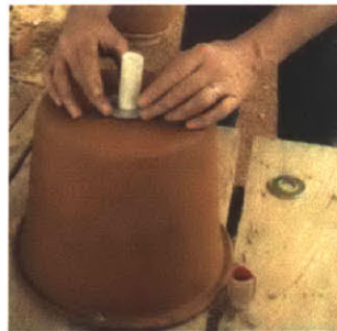
Gluing the steel water to the ceramic filter, held in alignment by the PVC pipe
