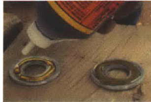
Applying Gorilla glue to the washers and let to sit for 5 - 10 minutes
