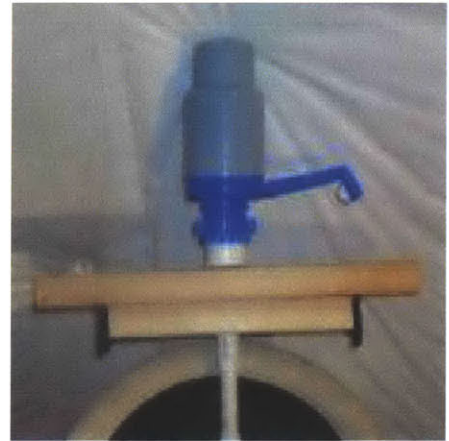
Figure 67 New design for wooden restraint to keep the KWK submerged Source: Chris Schulz
