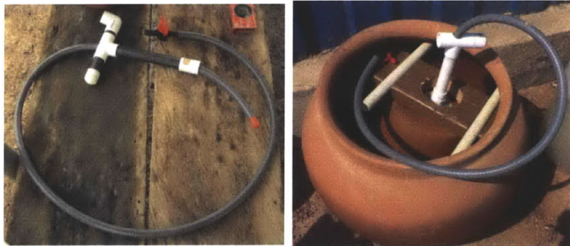
Figure 21 (left) Siphon Tube With Check Valve and Spigot Attached (right) Siphon Tube Installed in KWK
