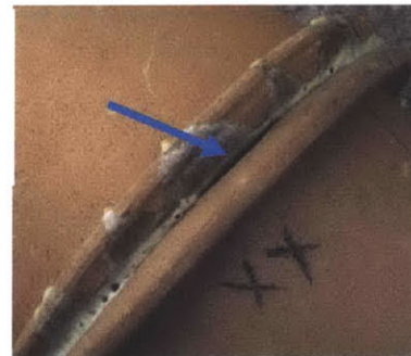
Figure 29 Hole in Seal Due to Gorilla Glue Failing to Expand
