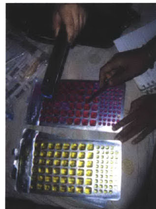
Figure 36 Counting Quanti-Tray™ Results
