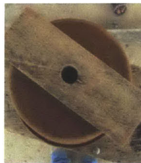
Wood guide to keep the drill stable
