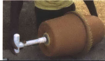
Screwing the T-joint handle to the top with the keg on its side
