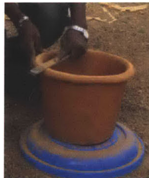
Filing the filter rims flat
