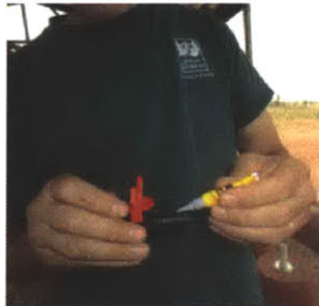
Applying superglue to shutoff valve
