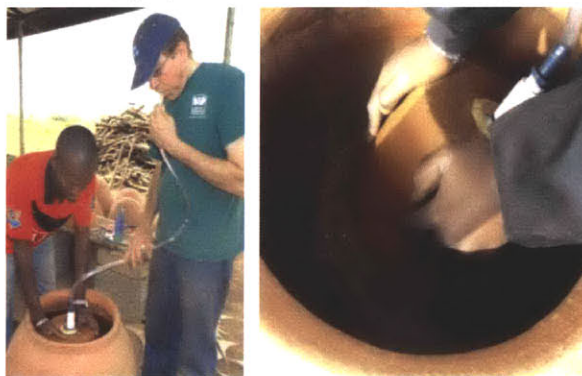
Figure 54 (left) Blowing into KWK for Leak Test and (right) Air Bubbles Escaping Through Leaks
