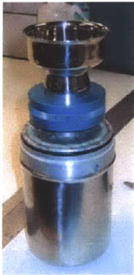
Figure 35 Membrane Filtration Field Unit
