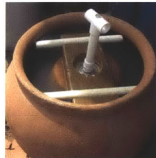
Figure 50 KWK Submerged with Wooden Restraint System
