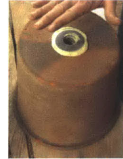
Figure 18 Metal Washer Sealed to the Ceramic Pot Filter Opening
