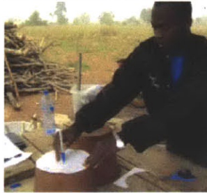
Marking off the center of the ceramic filter
