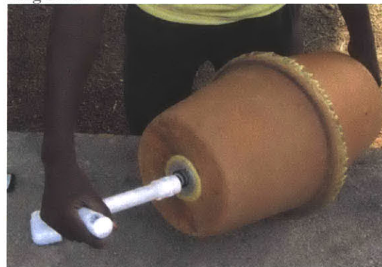
Figure 42 (top left) PVC Pipe With Holes Drilled In (bottom left) PVC Pipe Being Re-Threaded (bottom right) Screwing in PVC Riser Pipe with O-Ring Seals
