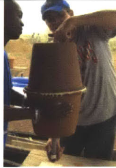
With an O-ring at the bottom, pushing the PVC pipe through keg
