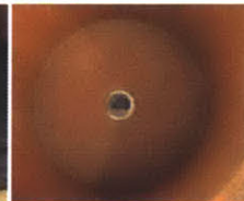
Removing the excess glue on top of the metal washer but leaving alone the glue on the ceramic
