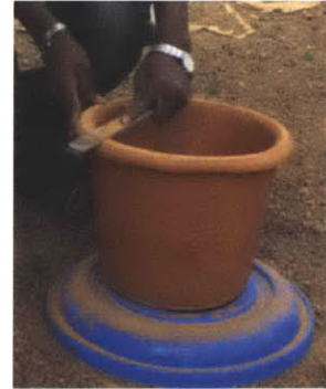
Figure 45 Filing Down the CT Filter's Rim
