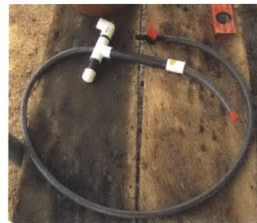
Figure 49 Siphon Threaded Through T-Joint
