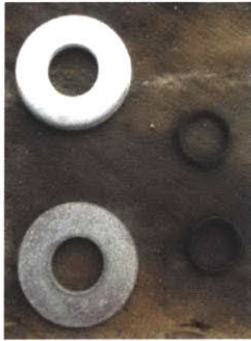
Figure 19 Metal Washers and O-rings Used to Create Seal at Keg/PVC Pipe Interface
