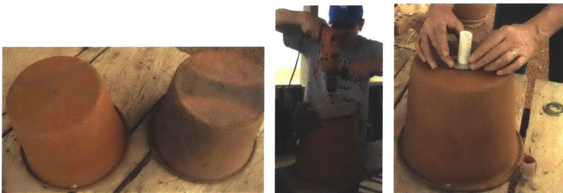
Figure 40 (left) Center Marked on CPFs (center) Hole Drilled Into Center of CPF (right) Metal Washer Sealed Around Hole
