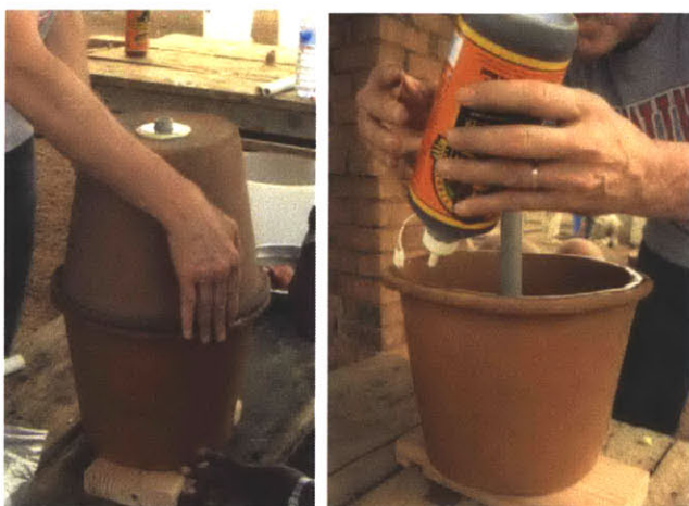
Figure 41 (left) Best Alignment Found to Match Up the CPFs (right) Gorilla Glue Applied to Rim
