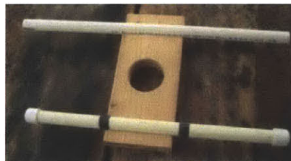
Top PVC pipe can slide left and right, but the bottom, with friction tape on, is held still
