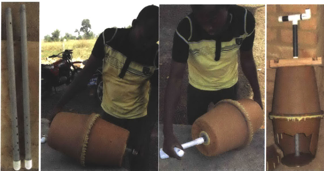
Figure 17 (left) PVC Riser Pipe and Its Installation (right) Broken KWK Shows Location of PVC Pipe
