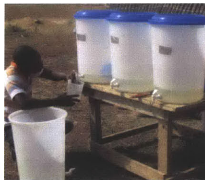
Figure 38 Measuring Volume Filtered by CPF
