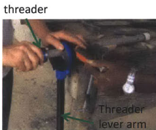
Threader Threader lever arm Threading the pipe – first by hand (left), and then using lever arm (right)
