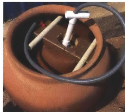
Figure 33 Wooden Restraint System Failing to Center KWK After KWK Fills With Water and Sinks
