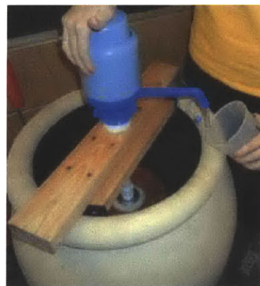
Figure 66 Water being removed from KWK with plastic hand pump Source: Chris Schulz
