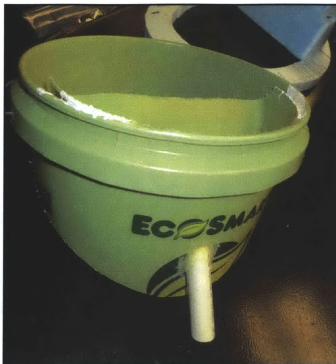
Figure 8-4 Prototype urine-separating toilet-seat using a bucket (side view) (Photo Credit: Mette Andersen)
