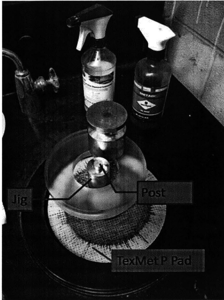
Figure 3-1: Polishing equipment used in step 1.
