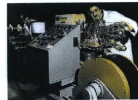
Fig.21-2: hot melt (or solvent) prepeg machine
