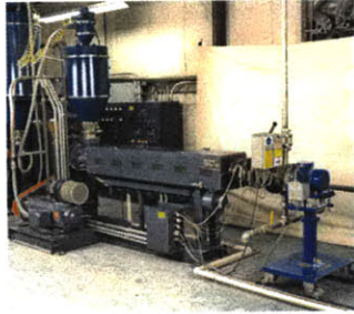
Fig.13-1: Merritt Extruder (polyurethane production for medical use)
