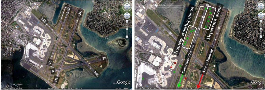
Figure 3-1: (Left) Layout of Boston Logan International Airport. (Right) Visualization of airport operations. Aircraft in green are departures and the ones in red are arrivals. A previously arrived aircraft can be seen at the bottom of the picture, waiting to cross the departure runway on the way to its gate.
