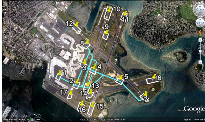
Figure 4-1: Layout of the airport surface at Boston Logan. Nodes in the network model are marked with white boxes. The configuration-specific network for departures from Runway 33L has been highlighted.
