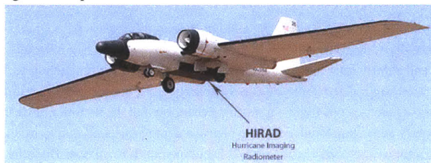
Figure 4.9: WB-57 high-altitude research aircraft. The WB-57 can carry up to 6,000 lbs for 6.5 hours at an altitude of 60,000 ft for a 2,500 nm range. Instruments are easily integrated onto the WB-57 due to its standard wing pods and manned configuration. (NASA ESPO 2010b)
