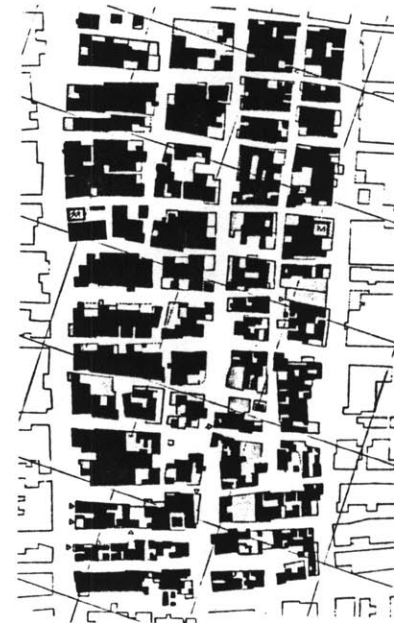
5-11 Detailed improvement area showing the incorporation of existing morphology within the new subdivisions
