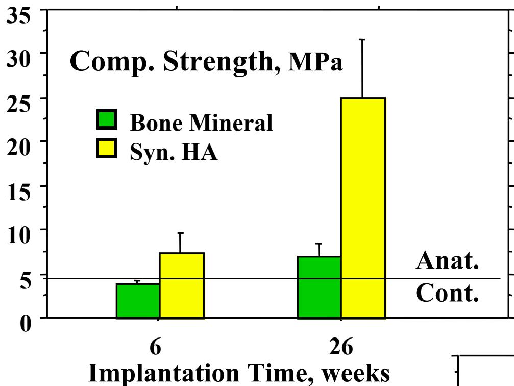
The strength of the site implanted with syn. HA is high but so to is the modulus (stiffness); bone mineral may provide adequate strength while having a near-normal modulus.
