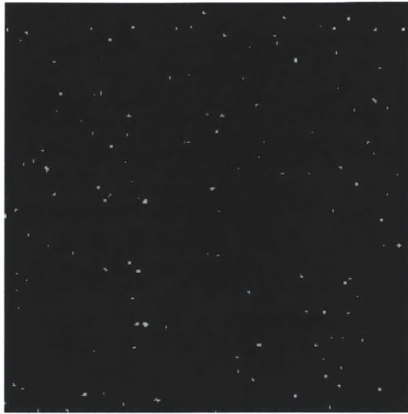
Figure 2-5: Zoomed view (250 x 250 pixels) of the thresholded refocused image from figure 2-3(b) revealing the particles and removing the background noise.
