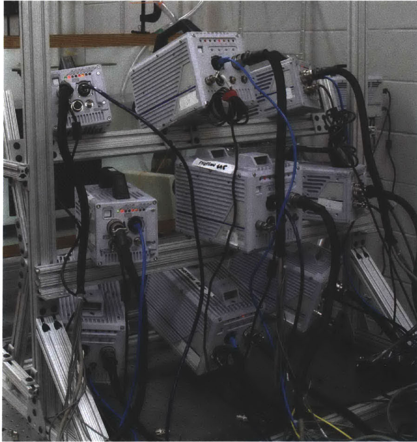
Figure 5-4: Arrangement of nine high speed Photron Cameras on a custom 80/20® frame.
