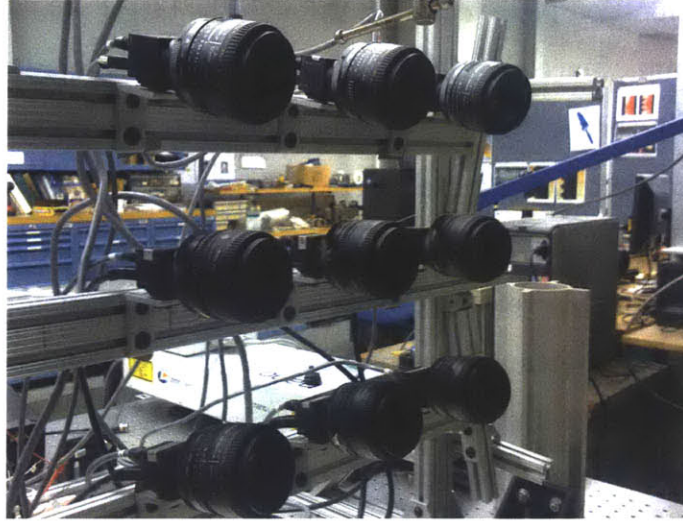
Figure 2-13: Photograph of the camera array. Nine cameras are mounted with 50 mm lenses on an extruded aluminum frame. Only eight cameras are used in the study.
