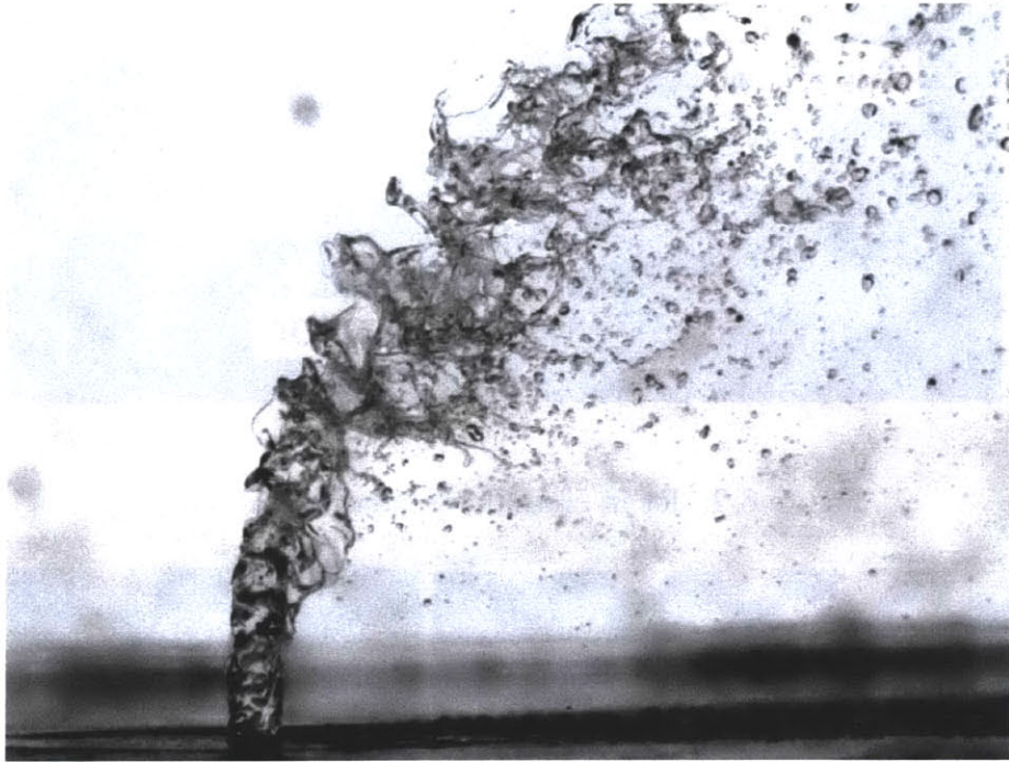
Figure 6-4: Raw image of liquid jet in cross-flow.
