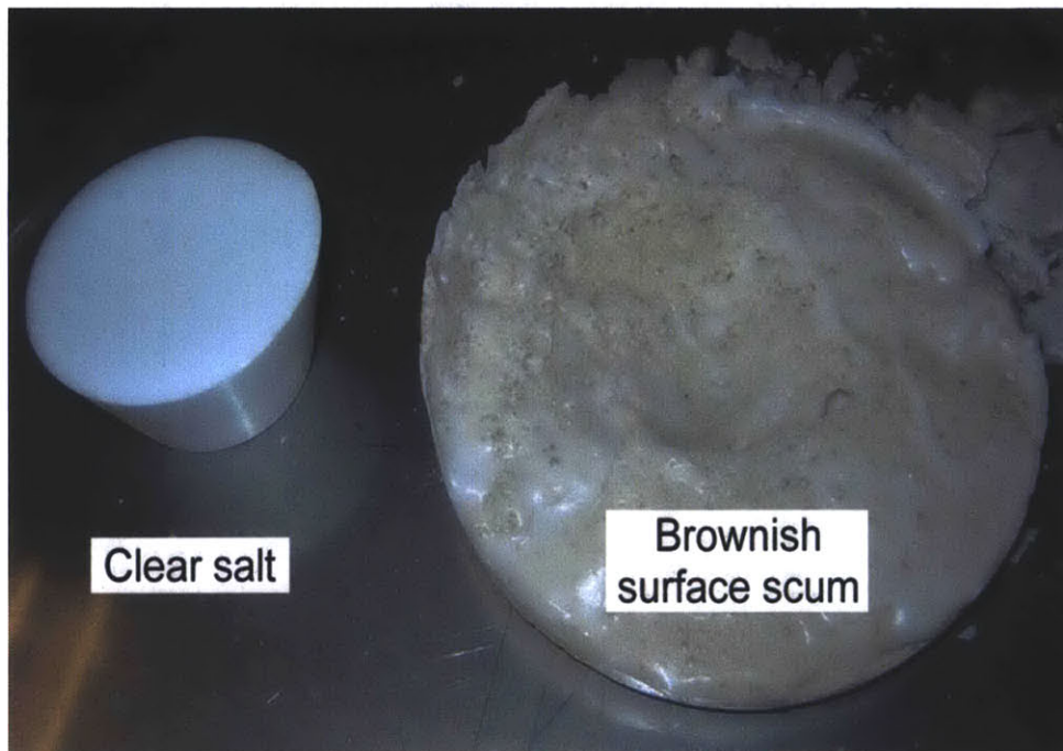
Figure 4.25 - Solidified pure and surface scum salt samples
