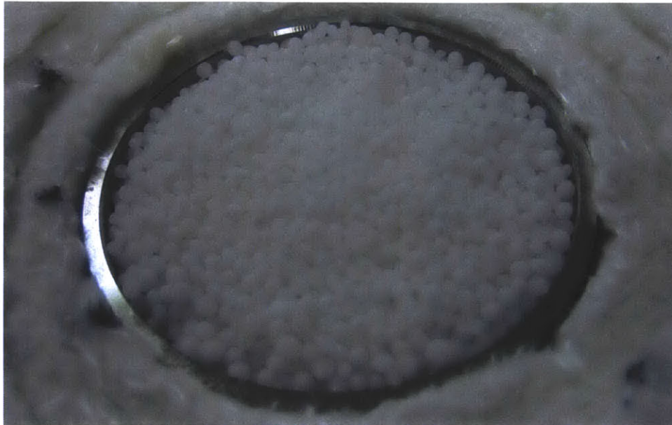
Figure 4.22 - Appearance of unmelted solar salt used in tests “Prilled” (pre-mixed) pellets, 1-3 mm diameter.
