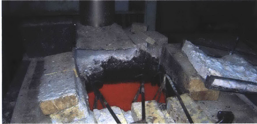
Figure 2.15 - Side draft fume hood used to collect salt vapors Fume extractor at rear of 600 °C tank with condensed salt buildup (Picture taken at Metallurgical Solutions, Inc. in RI)
