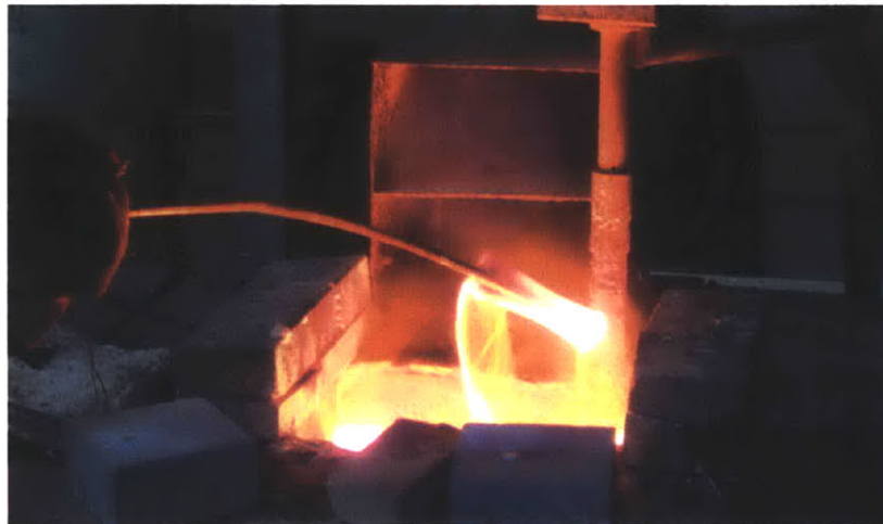
Figure 2.14 - Open air NaCl-KCl salt bath at 900 °C for metal heat treating (Picture taken at Metallurgical Solutions, Inc. in RI)
