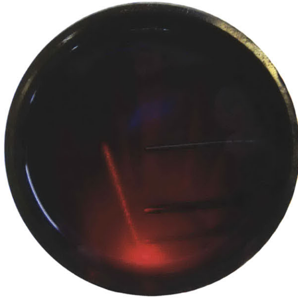
Figure 4.3 - Molten nitrate solar salt mixture in single tank test receiver
