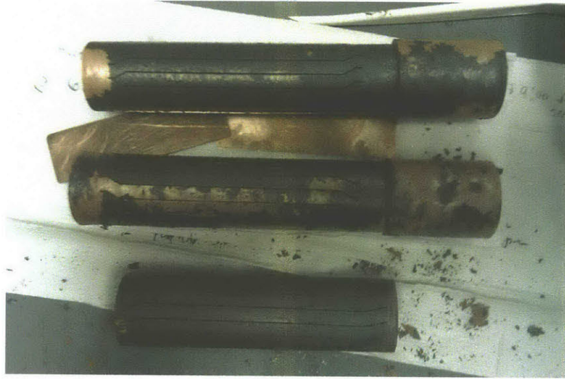
Figure 4-16: The top cylinders are oxidized in an attempt to create an insulation layer. However, the oxide layer was flaky and unreliable as an insulation. The bottom picture is a Paralyene coated cylinder.
