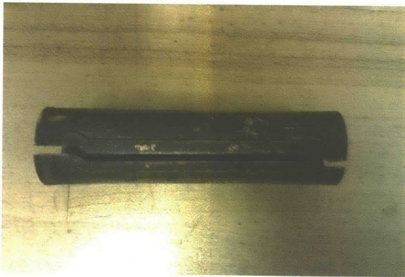
Figure 4-18: Ideally, the insulated inner cylinder can be inserted into the insulated outer cylinder. However, if necessary the outer cylinder can be split along one of the slits to create more clearance.
