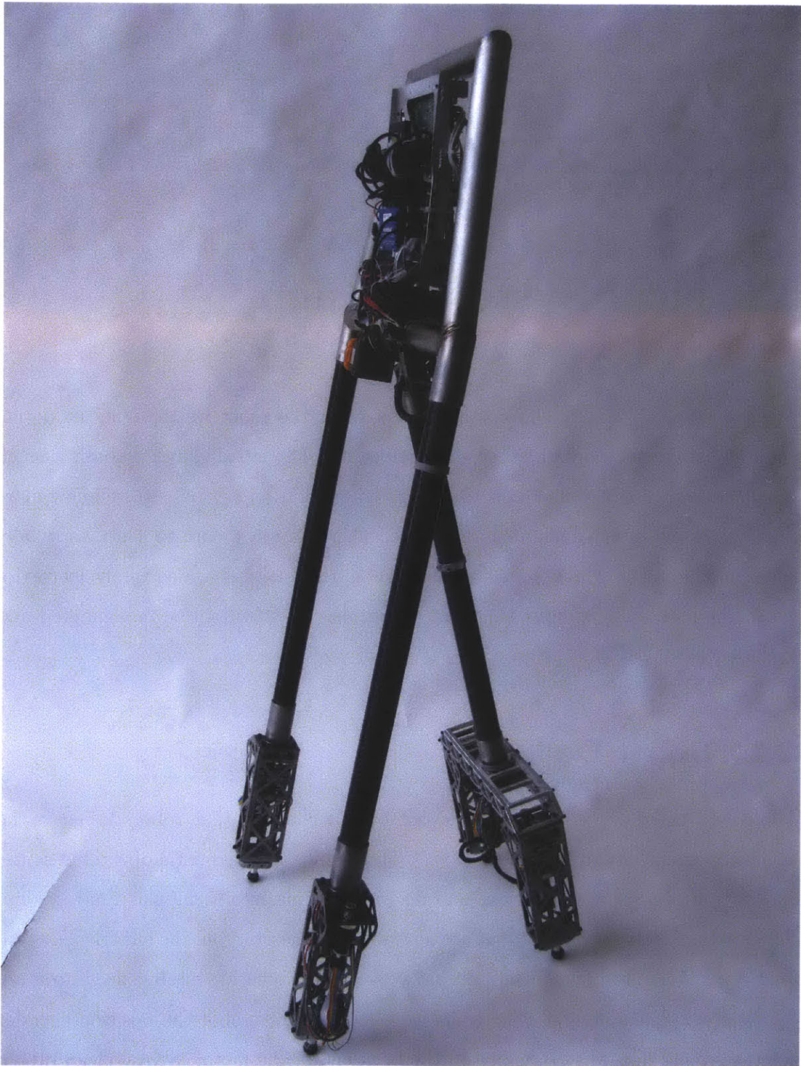
Figure 2-1: The full robot, a free walking realization of the simple compass gait model with a body. The robot is a planar walker but has three legs and four feet, with good reason.
