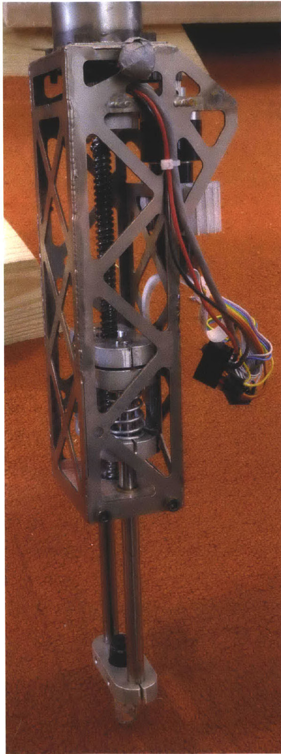
Figure 2-8: The robot's series elastic foot actuator.
