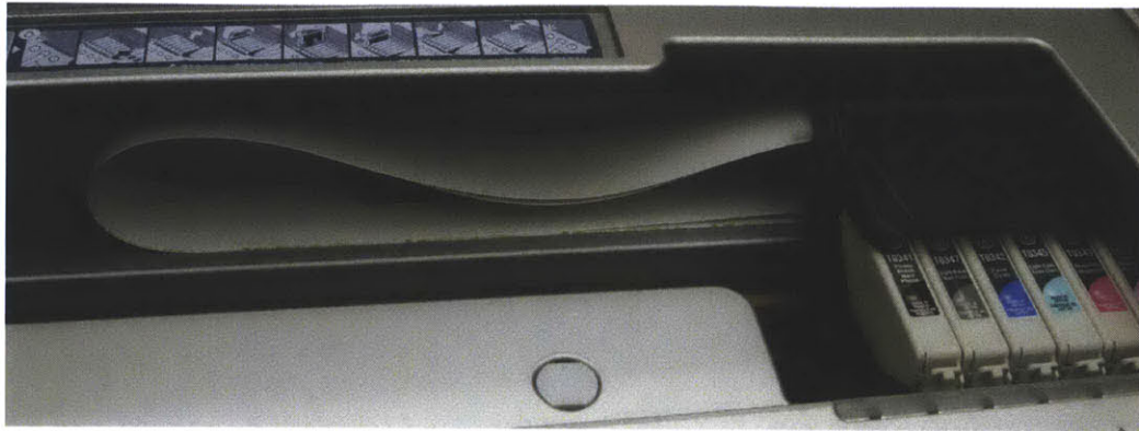
Figure 2-9: The cable which connects to the moving carriage in an inkjet printer was the design inspiration for the similar mechanism in the robot's feet.
