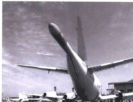
Figure 1: Magnetometer installed on the back of a P-3C aircraft for MAD 1
