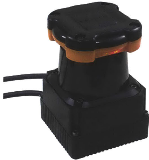
Figure 2-3: Image of the Hokuyo UTM-30LX scanning laser range finder.
