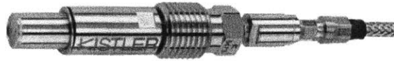
Figure 2.12. The pressure transducer used to measure the in-cylinder pressure is the Kistler 615C model. It has a sensitivity of 13.7 pC/bar with a linearity of \pm 0.5\% of the full scale.
