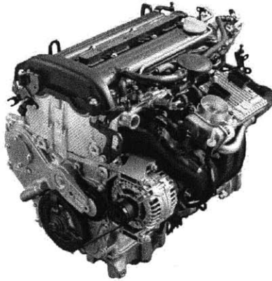
Figure 2.1. The DI version of GM Ecotec 2.2L was used in European GM models (Opel Signum, Opel Vectra) in early 2000's.
