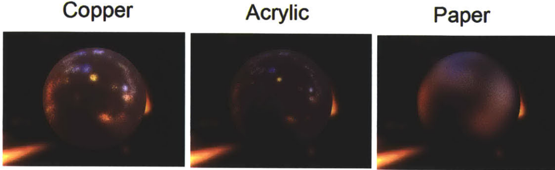
Figure 5-12: We obtain parametric fits for three different materials using the fast camera setup and render the results to compare them with each other. The figures show the rendered results and 1-D plots of the parametric model against half-angle. (a) Rendered result for Copper and its parametric fit. (b) Rendered result for Red Acrylic and its parametric fit. (c) Rendered result for Paper and its parametric fit.
