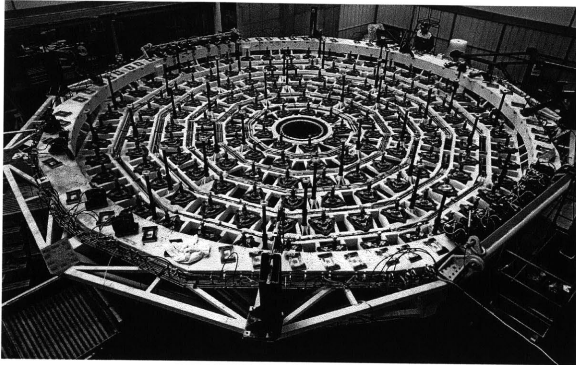
Figure 1-6: Mirror Support Structure for ESO 8.2-meter Telescope. Active supports are visible sticking up from the backplane. Observe the large number of degrees of freedom in the active support structure. Image Credit: ESO [12]
