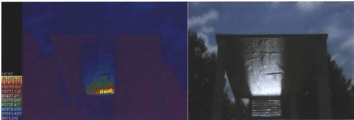
(b) 12' (3.66 m) from Facade, Peak Luminance: 260,000 cd/m 2
