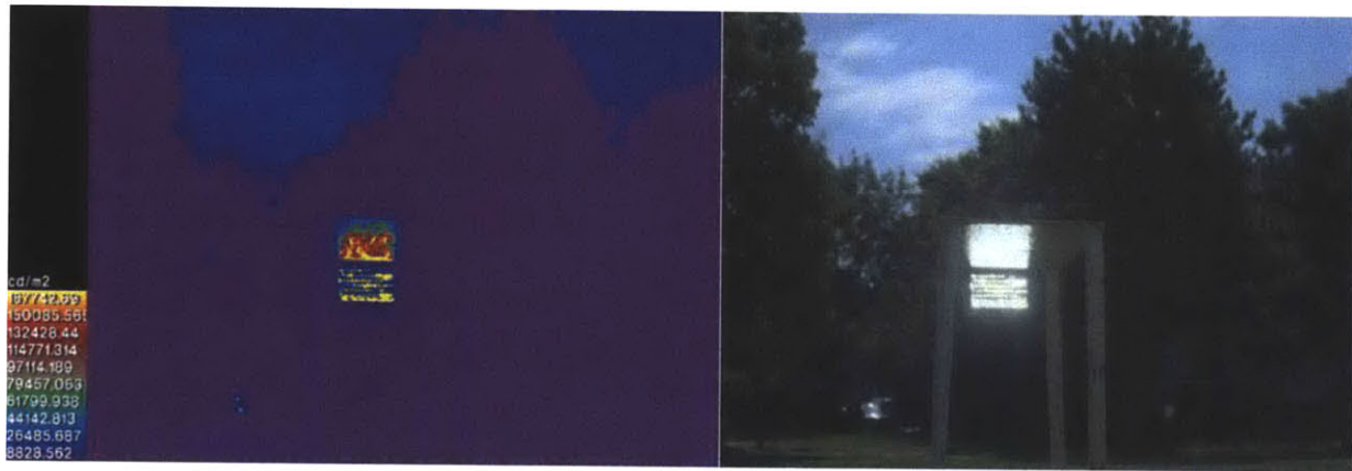
(b) 24' (7.32 m) from Facade, Peak Luminance: 220,000 cd/m 2
