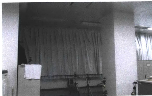
Figure 6.20: View of Mockup Office with All Curtains Drawn to Take Baseline Illuminance Measurements
