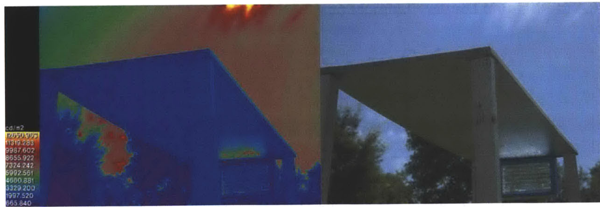
(c) Day 1, 12' (3.66 m) from Facade, 3' (.91 m) from Centerline, Peak Luminance on Ceiling Centerline: 6,000 cd/m 2
