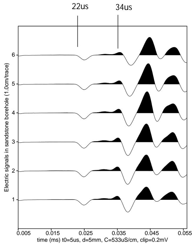
Figure 2: Seismoelectric signals recorded in the borehole in Figure 1. The amplitude in Figure 2a is normalized for each trace by  $200 \mu\text{V}$ . The fracture aperture is 5 mm. The conductivity of the saturant water is about  $0.533 \text{ mS/cm}$ .
