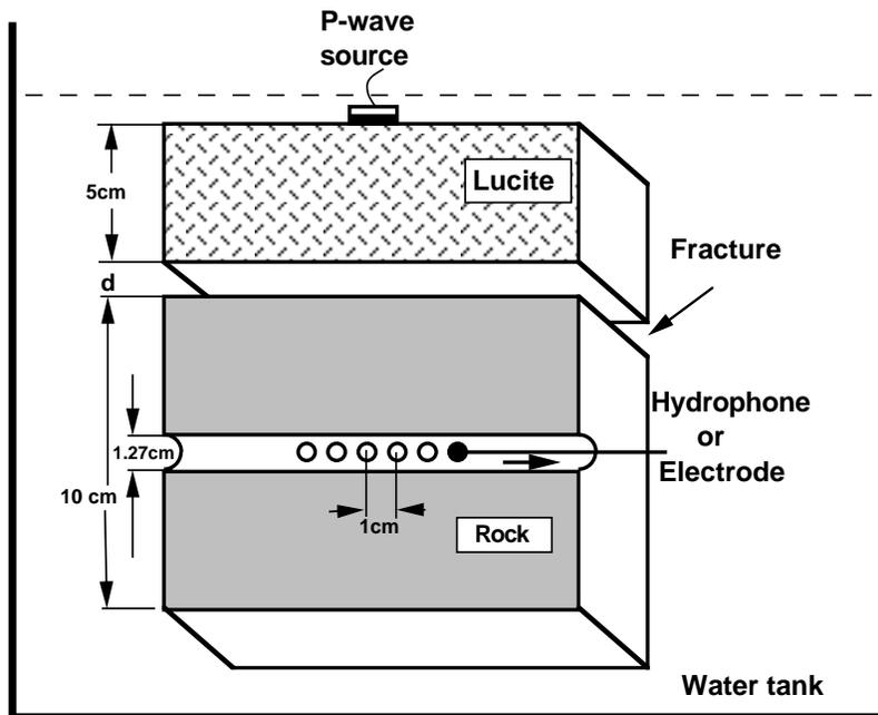
Figure 1: Borehole model with a fracture between rock and Lucite blocks. The model is saturated with water. A plane transducer is fixed on the Lucite block and generates an acoustic wave. A hydrophone or an electrode moves in the borehole and records the acoustic or electrical signals.
