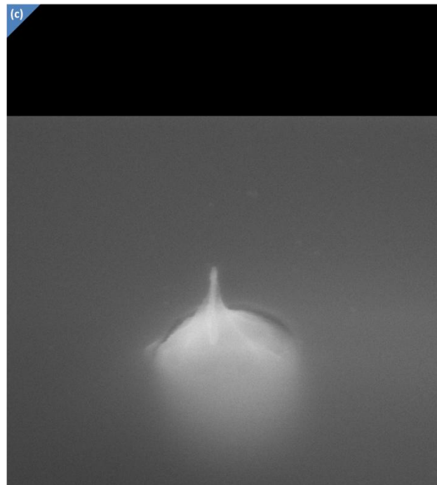
Figure 4-17: Turning the non-conformality of the resist coating process to advantage, the SiO 2 encasing the top of the CNT can be removed with HF whilst protecting the underlying release layer with photoresist. The process is shown schematically in (a), with SEMs from before (b) and after (c).
