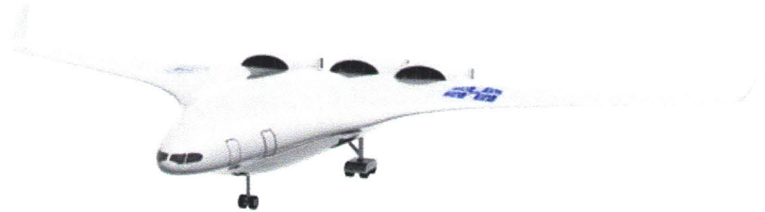
Figure 1-1: The Silent Aircraft Initiative SAX-40 featuring boundary layer ingestion and embedded propulsion systems.
