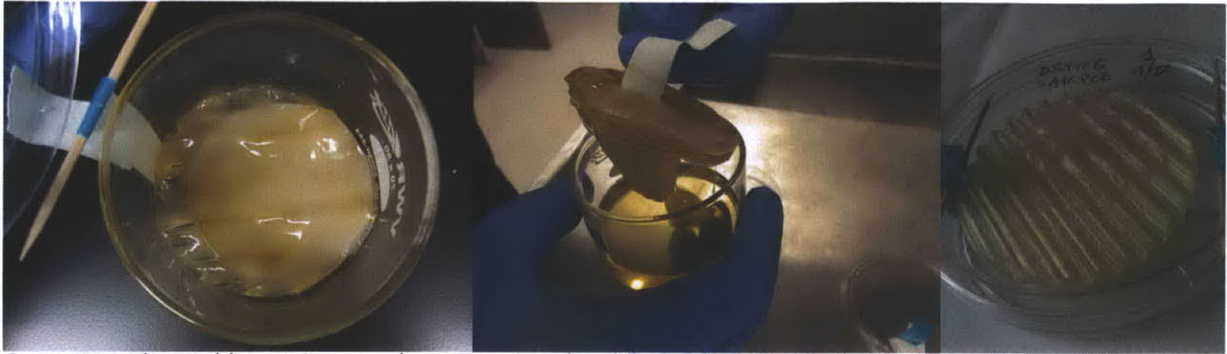
Grow-around-a-mold experiment, where 3D printed molds were inserted in the liquid medium and the bacteria grew cellulose structures around the molds.
