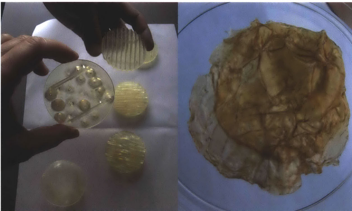
Left: variety of 3D printed molds used to test the conformational capacity of the cellulose structures. Right: Cellulos pellicle being extremely thin when dry, remains elastic and deforms inevitably when de-molding, retaining only partial aspects and features of the molded shape.
