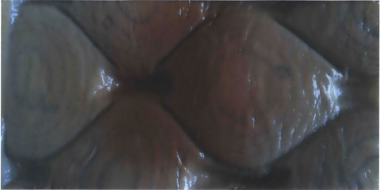
Thick wet pellicle applied over a dry mold in order to test conformation of the pellicle to a mold.
