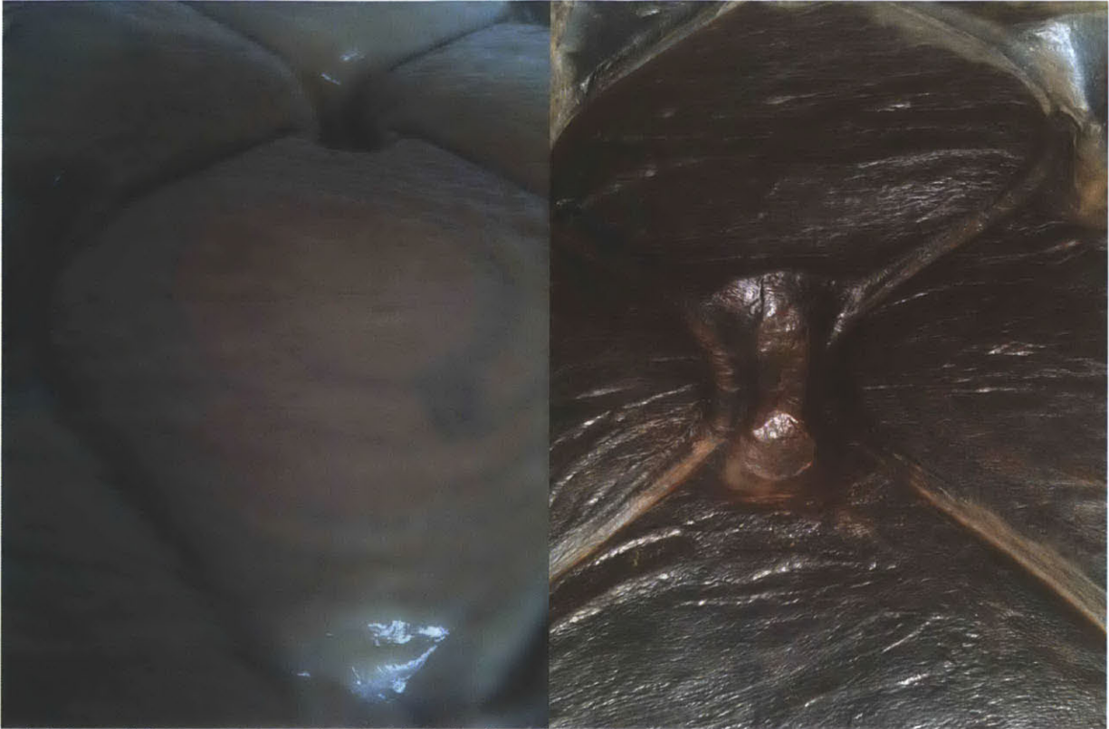
Left: Wet pellicle over CNC wooden mold. Right: dry pellicle after being demolded.
