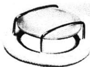
Figure 4: The Kay-Shiley flat-disc valve design.
