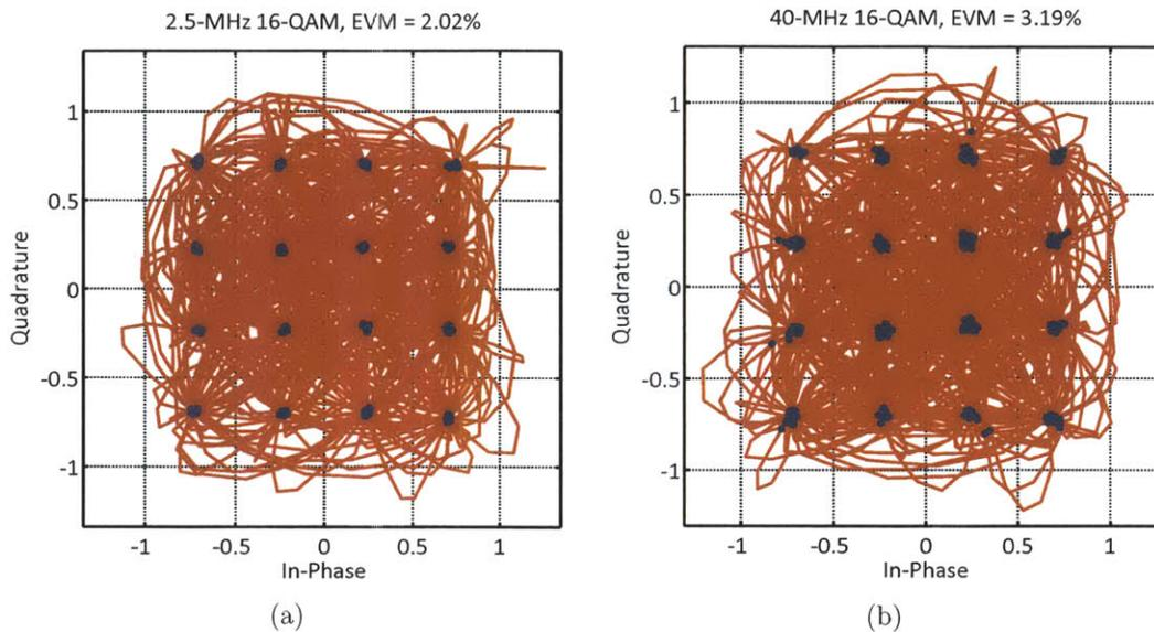
Figure 4-43: Constellation diagram of a 16-QAM signal transmitted by the AMO system at 2.5 MHz and 40 MHz symbol rate for the 1.95-GHz AMO transmitter. (a) 2.5 MHz. (b) 40 MHz.
