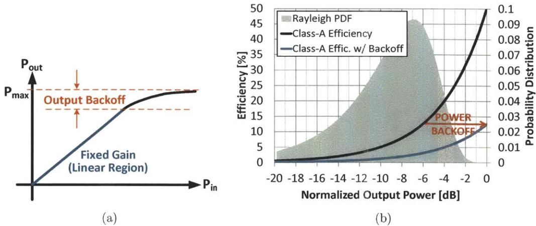
Figure 1-1: (a) Typical transfer characteristic for a conventional conducting-class PA. (b) Efficiency vs. output power for a class-A PA with and without power backoff. A Rayleigh output power probability distribution, which is a typical of many wireless communication standards today, is also shown for reference.
