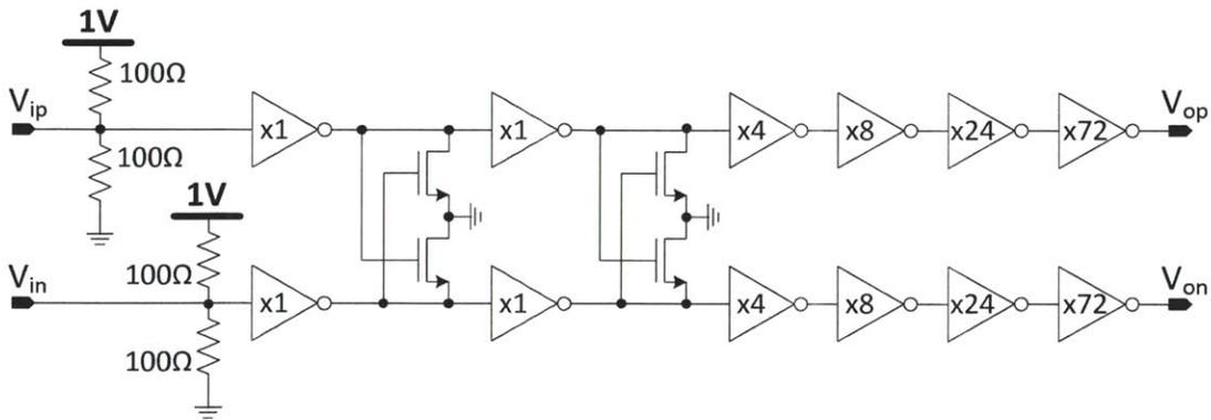
Figure 5-8: The differential PA input buffer that interfaces the off-chip RF phase input to the on-chip PA in the AMO IC prototype.
