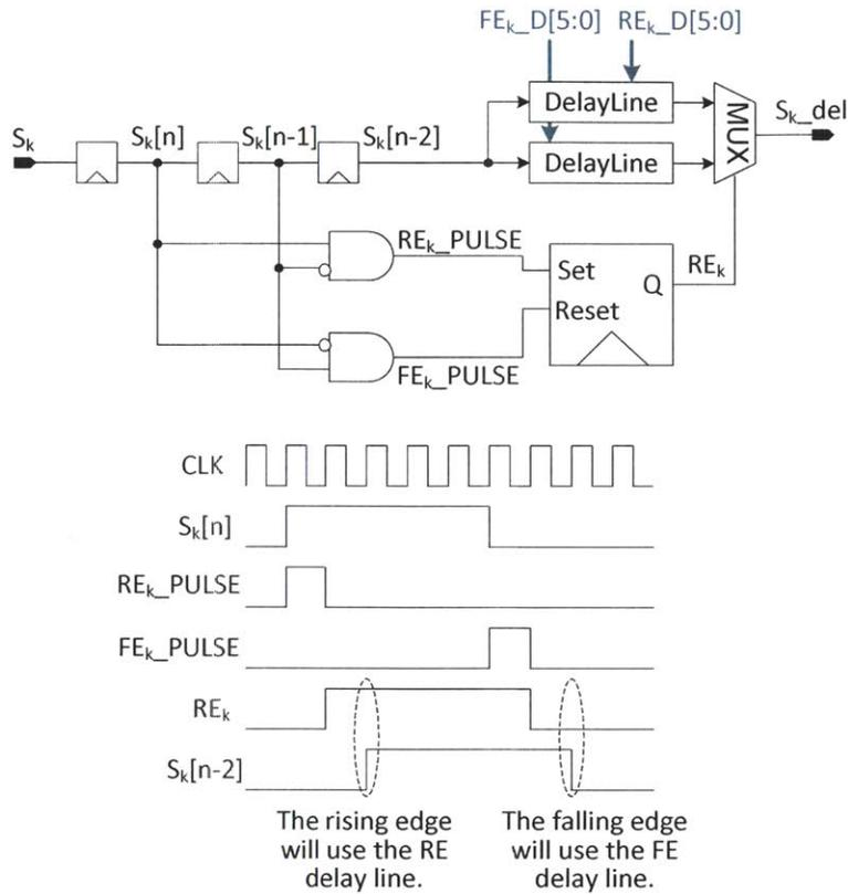
Figure 5-10: Block diagram and timing waveforms of the delay adjustment circuit used to tune the delay of the signal transitions for both rising edges and falling edges. The delay adjustment circuit implements time alignment between the different switches used in the 2.4-GHz AMO IC prototype.
