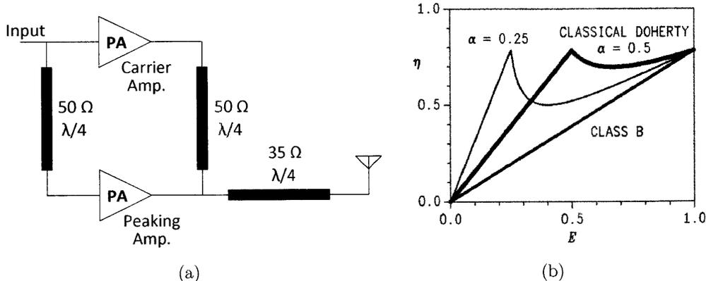
Figure 2-8: (a) Classical Doherty architecture. (b) Theoretical efficiency vs. normalized output amplitude for the classical Doherty architecture, for two different locations of the first efficiency peak. The efficiency of an ideal class-B PA is also shown for reference.
