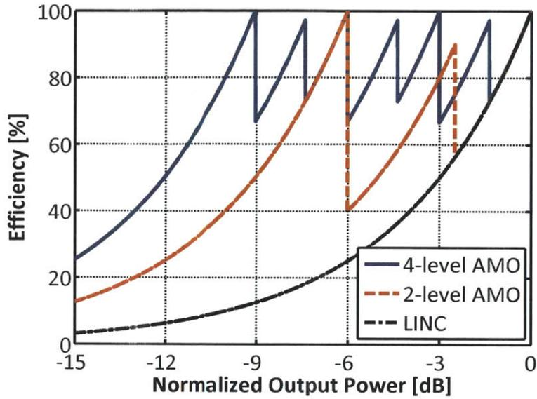
Figure 4-7: Efficiency vs. output power of AMO modulation when there are 4 amplitude levels available vs. when there are 2 amplitude levels available.
