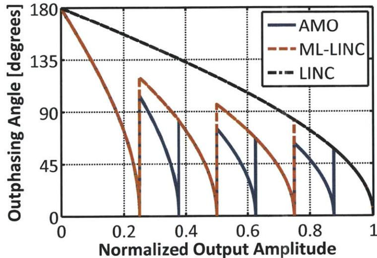
Figure 4-4: Outphasing angle vs. output amplitude of AMO modulation compared to LINC and ML-LINC, when 4 different PA amplitude levels are available. AMO always results in the minimum outphasing angle.
