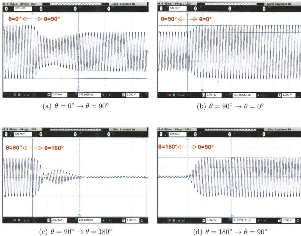
Figure 5-26: Measured step response of the 2.4-GHz AMO transmitter output envelope when the outphasing angle is changed with a fixed supply voltage. (a)  $\theta = 0^\circ \rightarrow \theta = 90^\circ$ . (b)  $\theta = 90^\circ \rightarrow \theta = 0^\circ$ . (c)  $\theta = 90^\circ \rightarrow \theta = 180^\circ$ . (d)  $\theta = 180^\circ \rightarrow \theta = 90^\circ$ .
