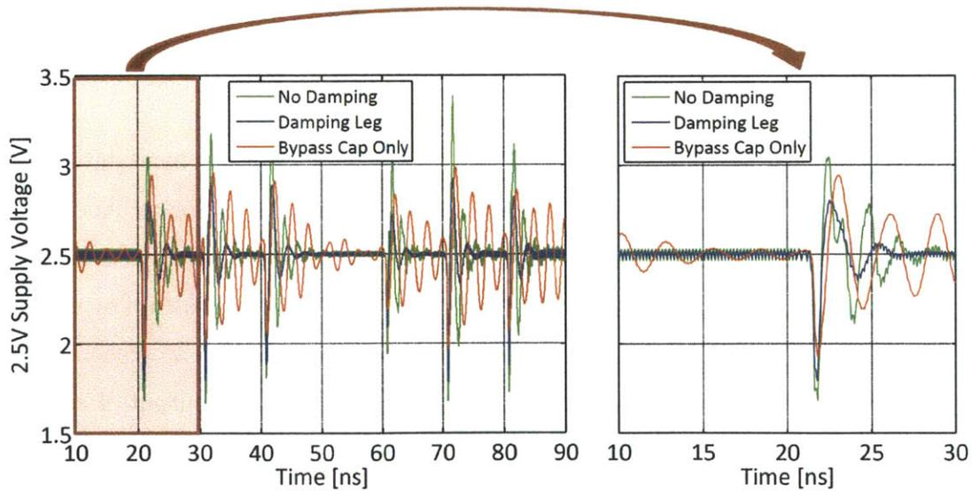
(b) Power Supply for Switch Buffers,  $V_{DD25}$
