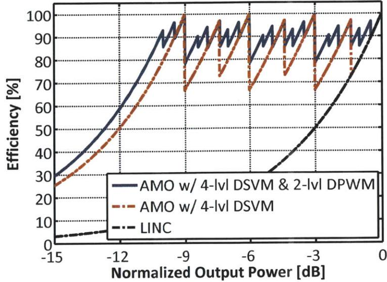
Figure 4-12: Efficiency of the AMO system using 4-level DSVM (red line) vs. the AMO system using 4-level DSVM combined with 2-level DPWM (blue line).
