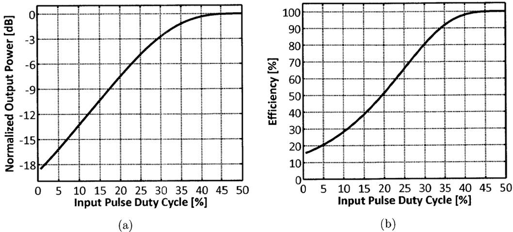
Figure 2-6: Output power (a) and efficiency (b) of an ideal class-E PA with various input duty cycles.
