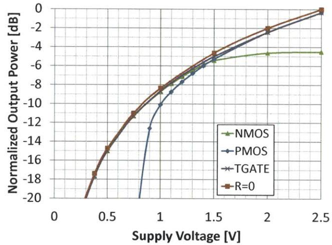
(b) PA Output Power vs. Supply Voltage
