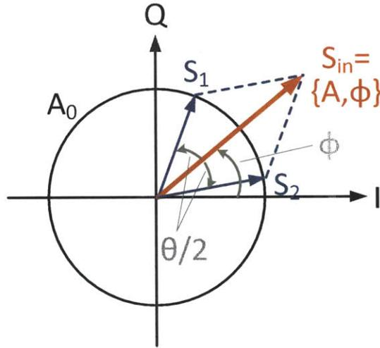
Figure 2-2: LINC vector diagram, including notational convention.
