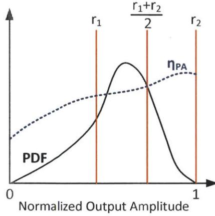
Figure 4-13: Example amplitude PDF for a signal (black line), along with an example PA efficiency curve  $\eta_{PA}$  vs. output amplitude (blue line). The  $r_k$  are the maximum output amplitudes for each of the different supply voltage levels  $V_{sup,k}$  when both PAs are driven by the same supply. There are 2 amplitude levels available in the example above.
