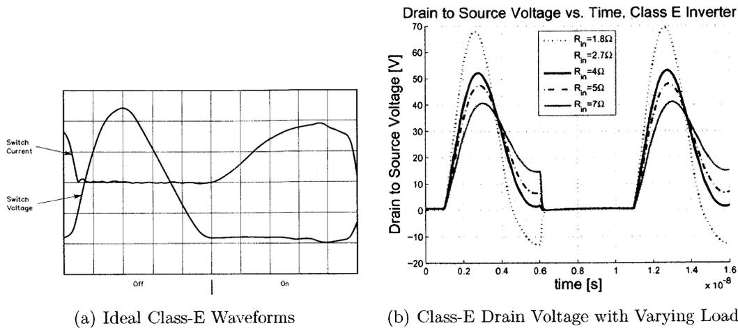
Figure 3-3: (a) Ideal voltage and current waveforms of the main transistor in a class-E PA. (b) The drain voltage waveform of a class-E PA for various values of load resistance.
