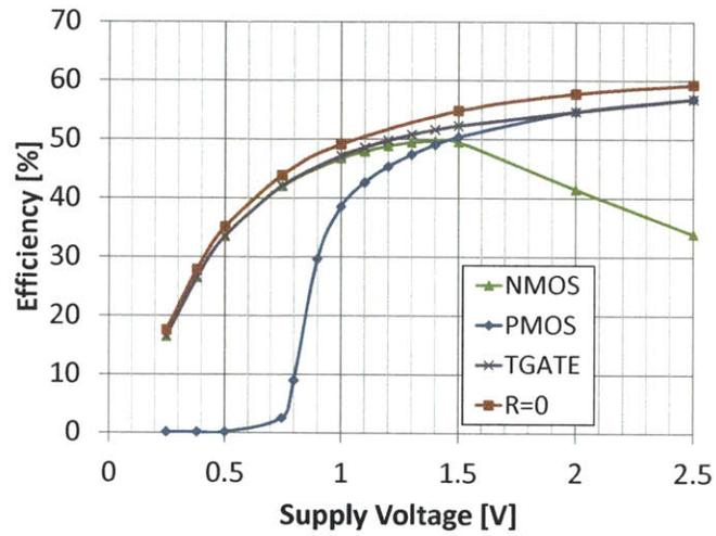
(a) PA Efficiency vs. Supply Voltage
