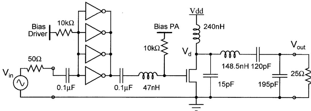
Figure 3-13: Circuit schematic of the class-E power amplifier used in the OPERA prototype.
