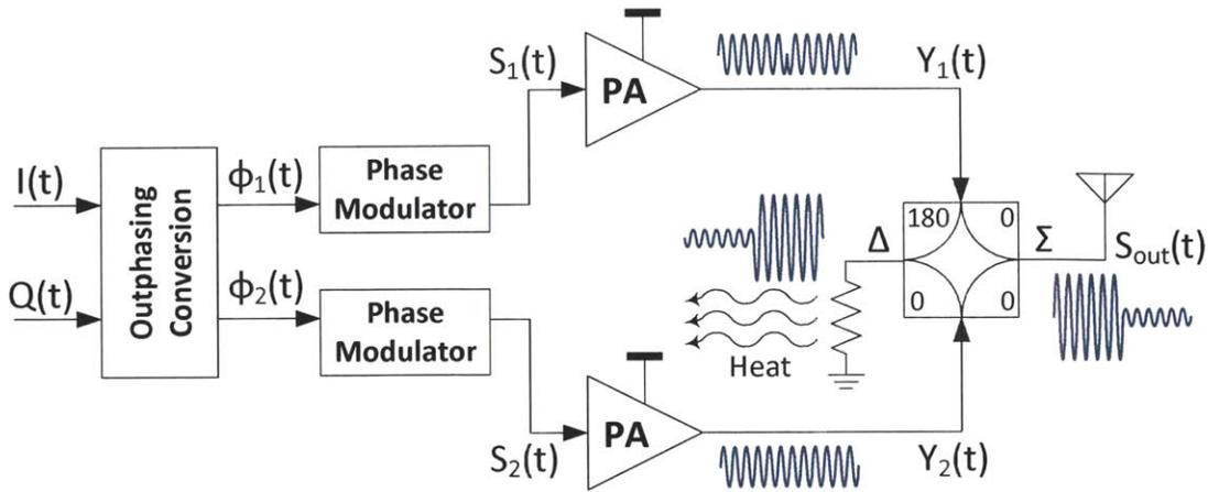
Figure 2-1: Conventional outphasing, or LINC, architecture.
