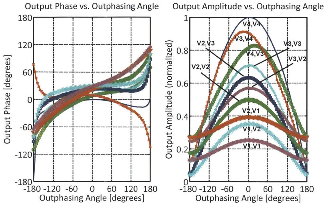
Figure 4-23: Measured output amplitude and phase vs. outphasing angle for the prototype AMO system with DPWM. Each curve corresponds to a different combination of discrete pulse widths for the two outphased PAs.
