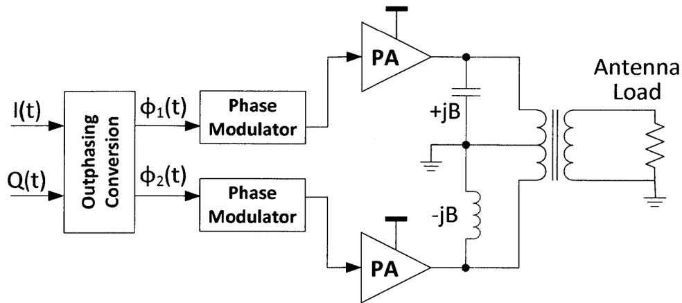
Figure 2-9: Chireix outphasing transmitter.
