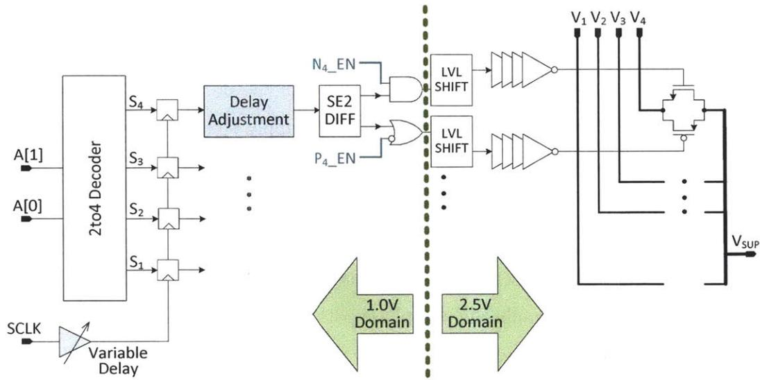
Figure 5-9: Block diagram of the discrete supply-voltage modulator used in the 2.4-GHz AMO IC prototype.
