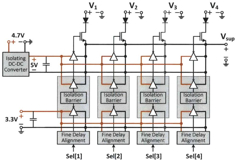
Figure 4-36: 4-level discrete supply modulator for the 1.95-GHz AMO prototype.
