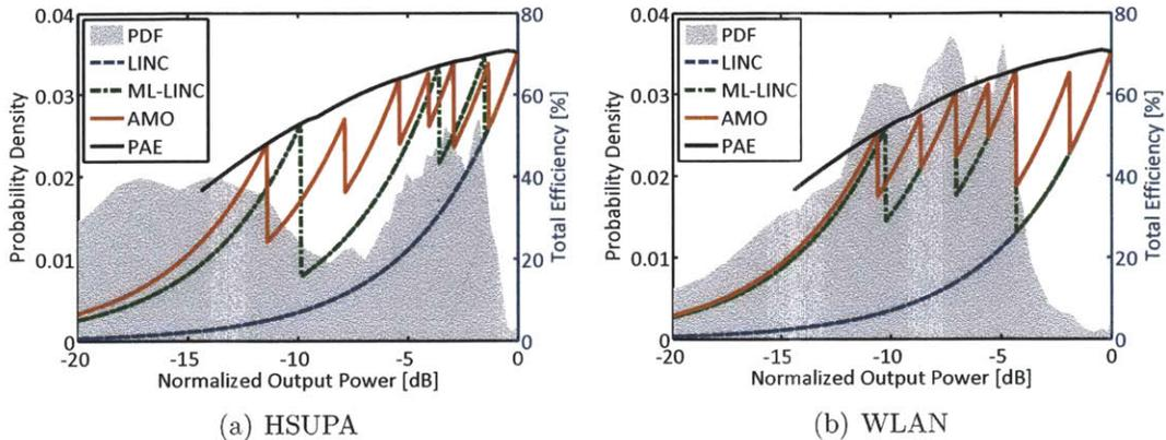
Figure 4-14: Amplitude PDF of a modulated signal and corresponding optimum efficiency curves for LINC, ML-LINC, and AMO with 4 available supply voltages. (a) HSUPA signal. (b) WLAN signal.
