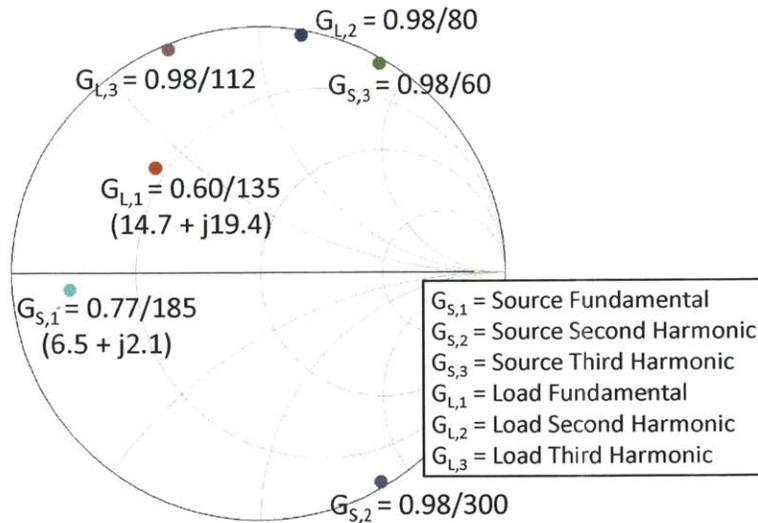
Figure 4-30: Optimum input and output impedances at the fundamental, 2nd harmonic, and 3rd harmonic of the RF carrier frequency for maximum efficiency for the class-E GaN PA.
