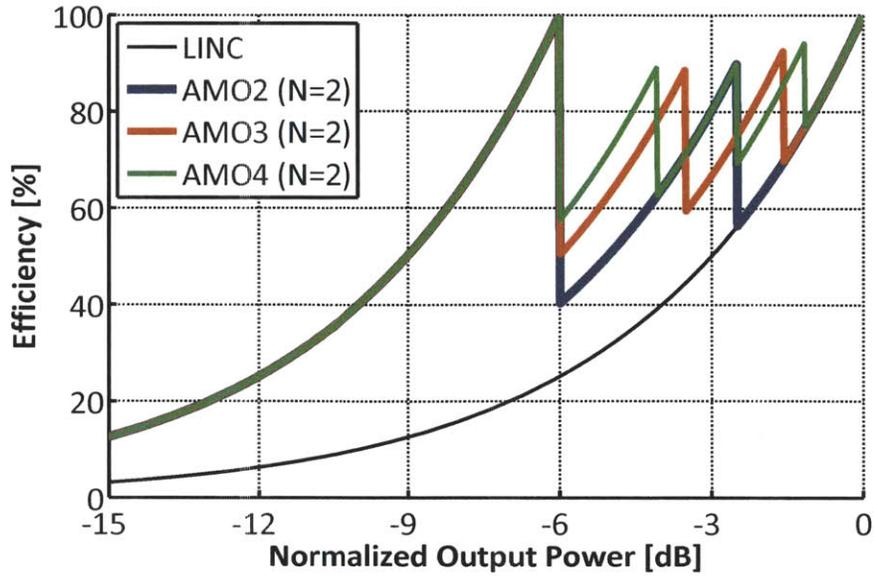
Figure 6-1: Theoretical efficiency for the AMO system using 2, 3, and 4 PAs. 2 supply voltages are available for each case, with the amplitude levels spaced 6 dB apart.
