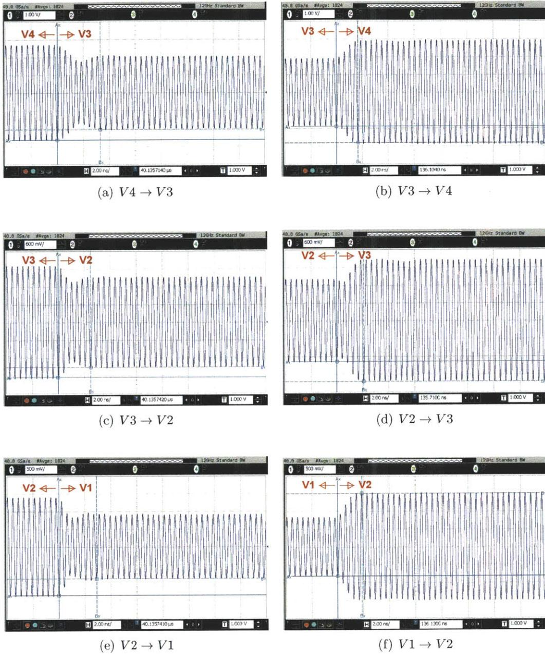
Figure 5-25: Measured step response of the 2.4-GHz AMO transmitter output envelope when the supply voltage is changed for both PAs. (a)  $V4 \rightarrow V3$ . (b)  $V3 \rightarrow V4$ . (c)  $V3 \rightarrow V2$ . (d)  $V2 \rightarrow V3$ . (e)  $V2 \rightarrow V1$ . (f)  $V1 \rightarrow V2$ .
