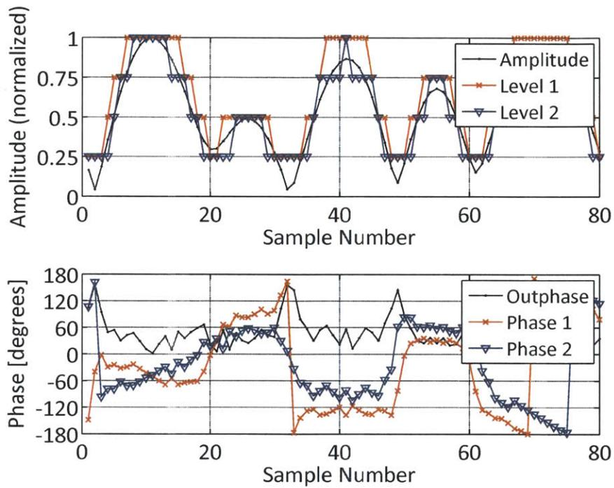
Figure 4-19: Time-domain waveforms of the PA amplitudes and phases resulting from the AMO signal decomposition with DPD,  $A_1$ ,  $A_2$ ,  $\phi_1$ ,  $\phi_2$ , for a segment of the 16-QAM signal shown in Figure 4-18(a), using the example measured data shown in Figure 4-15. The amplitude of the input signal and the outphasing angle between the two PAs is also shown.
