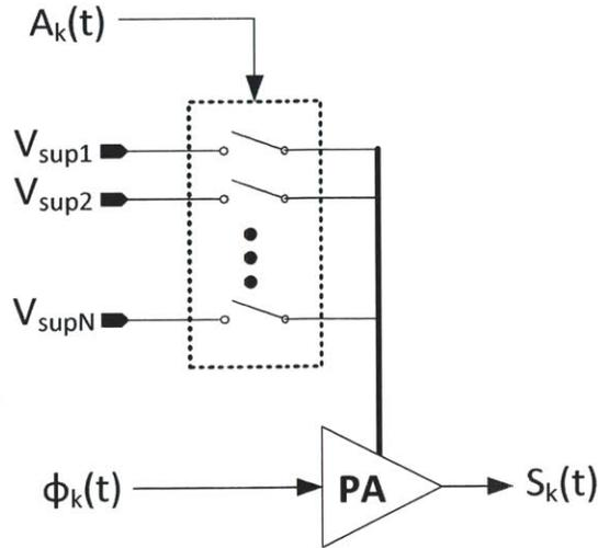
Figure 4-8: Example of a discrete supply-voltage modulator (DSVM).
