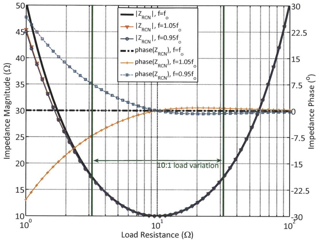
Figure 3-6: RCN impedance vs. load resistance for a frequency deviation of  $\pm 5\%$  of the center operating frequency.  $Z_o = X = 10\Omega$ .
