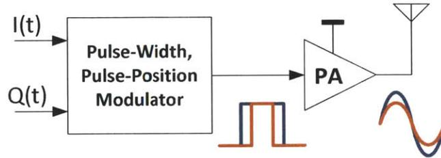
Figure 2-5: Pulse-width pulse-position modulated PA architecture.
