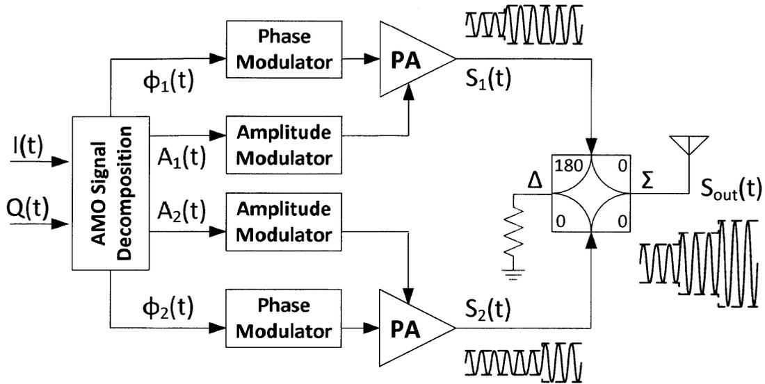
Figure 4-1: Asymmetric multilevel outphasing (AMO) architecture.
