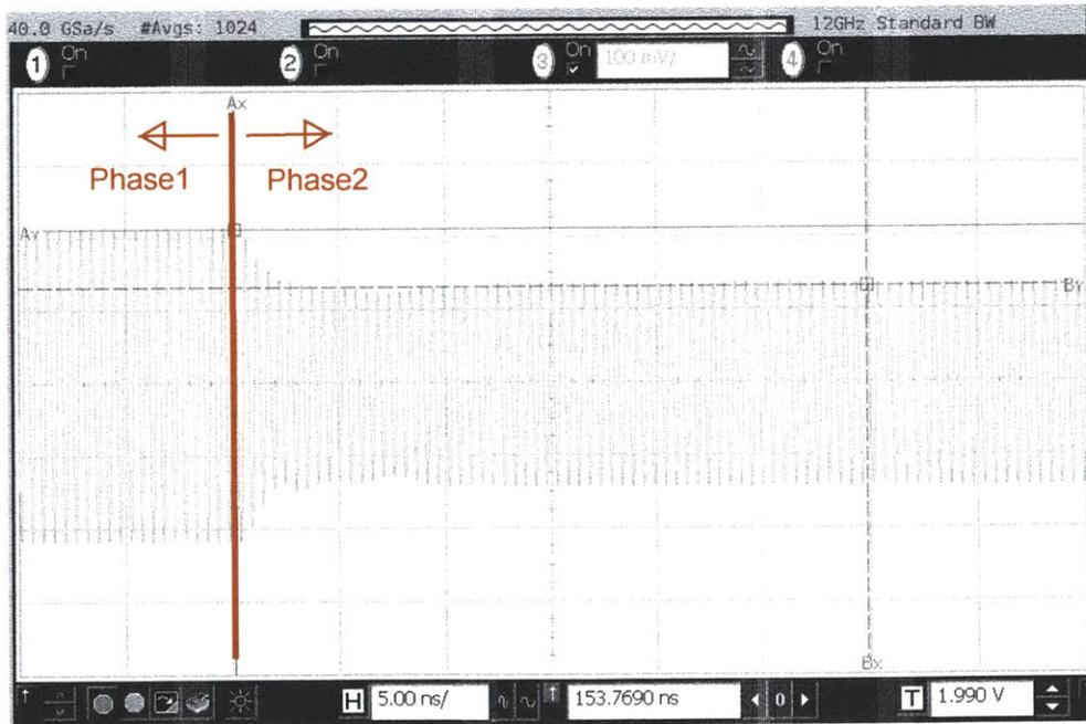
Figure 4-42: Measured step response of the 1.95-GHz AMO transmitter output envelope when the outphasing angle is changed from one value to another with a fixed supply voltage.
