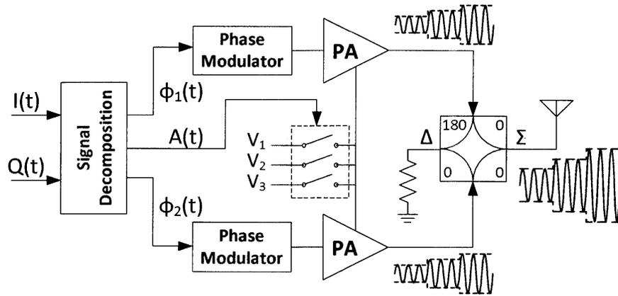
Figure 2-11: Multi-level LINC architecture. Three supply voltages are shown in the figure, but there can be any number of supply voltages greater than 1 for the ML-LINC system.
