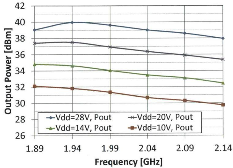
Figure 4-33: Measured output power vs. frequency at various supply voltages for the class-E GaN PA.
