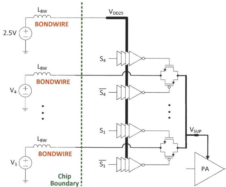
Figure 5-15: Interface between the external power supply voltages and the discrete supply voltage modulator on the AMO IC prototype, showing the parasitic series bondwire inductance that causes transient ringing on the on-chip supply voltage nodes.
