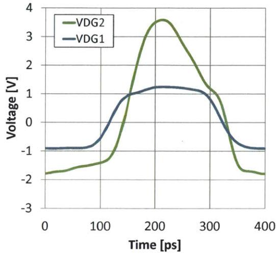
Figure 5-7: Simulated gate-drain voltages  $V_{DG2}$  and  $V_{DG1}$  across the thick-oxide CG device and the thin-oxide CS device, respectively, at the maximum PA supply voltage of 2.5 V.
