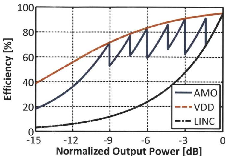
Figure 4-9: Efficiency vs. output power of the AMO system with DSVM when 4 different supply voltage levels are available, assuming a fixed power loss of -13dB relative to the maximum output power. The only other loss accounted for in the plot is the loss due to the asymmetric combining.
