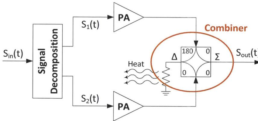
Figure 1-3: LINC system with conventional isolating combiner.
