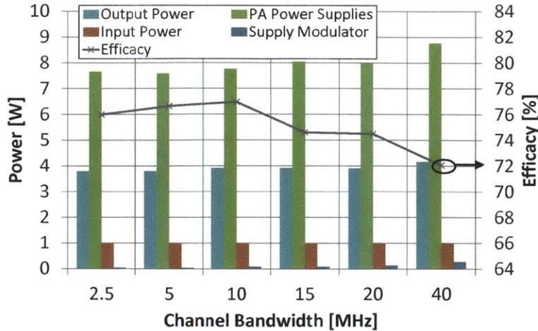
Figure 4-45: Power breakdown and efficacy of the 1.95-GHz AMO prototype for the 16-QAM signal transmission for various channel bandwidths.
