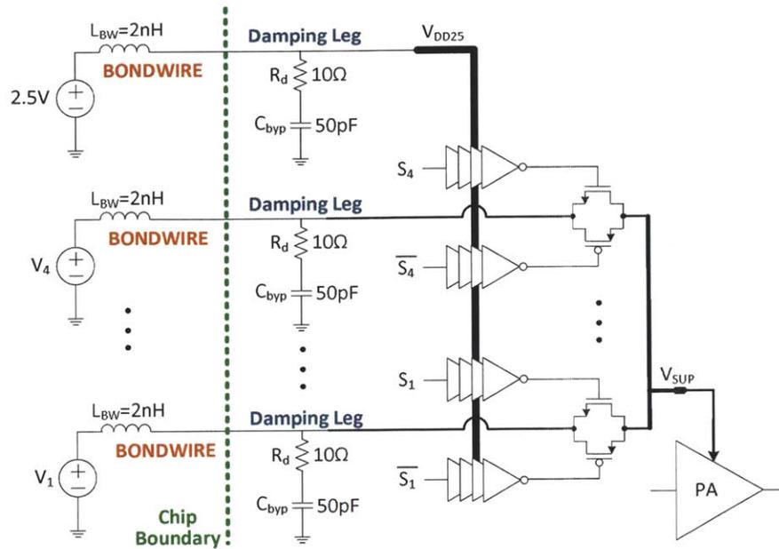
Figure 5-16: Discrete supply voltage modulator with damping legs to reduce the transient ringing on the on-chip supply voltage nodes in the 2.4-GHz AMO IC prototype.
