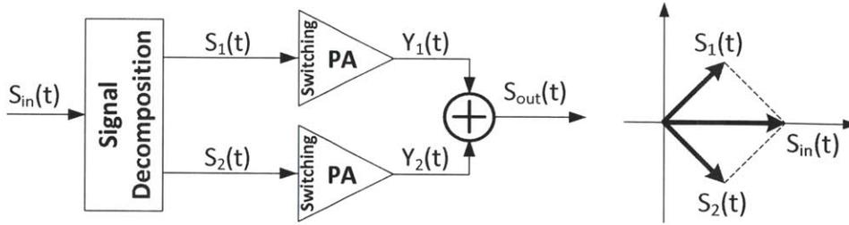
Figure 1-2: (a) LINC principle diagram. (b) LINC vector diagram.
