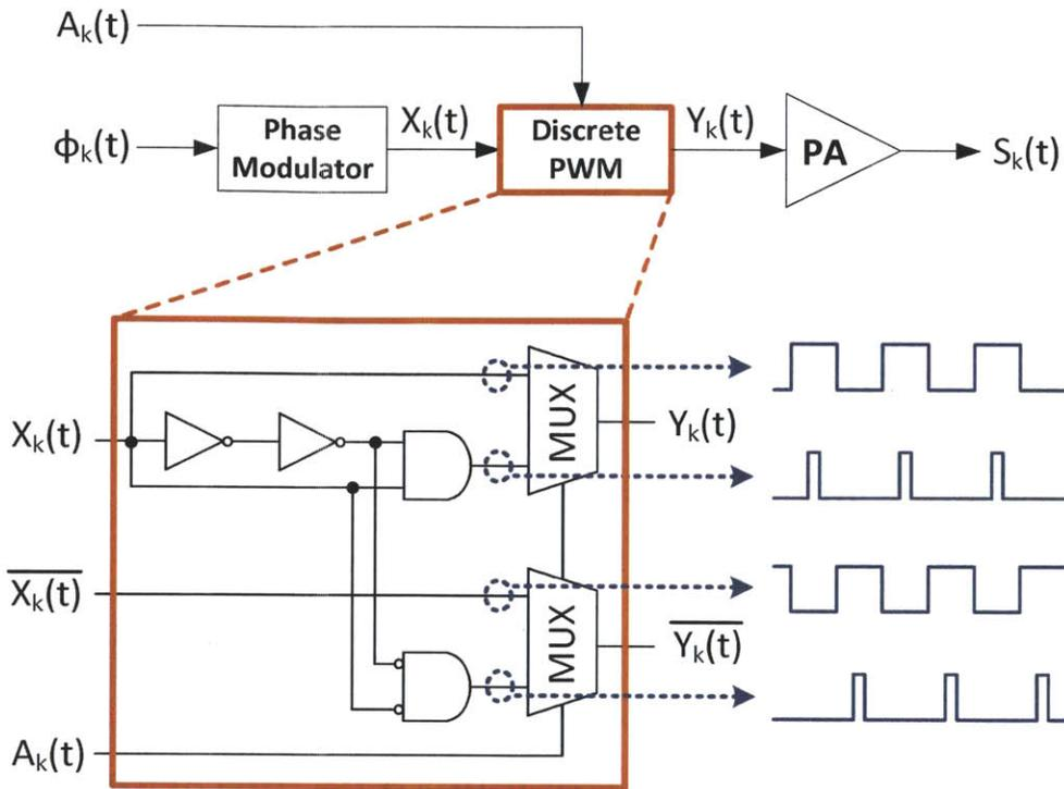
Figure 4-10: Example implementation of a 2-level discrete pulse-width modulator (DPWM).
