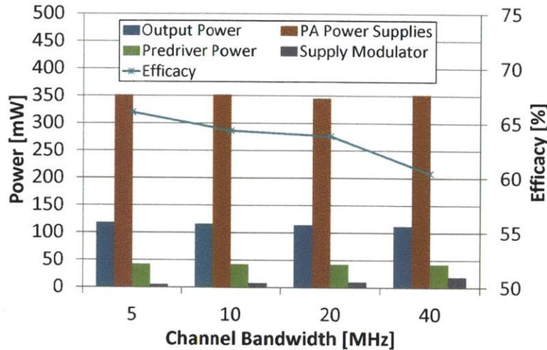
Figure 5-30: Power breakdown and efficacy of the 2.4-GHz AMO IC prototype for the 64-QAM signal transmission for various channel bandwidths.
