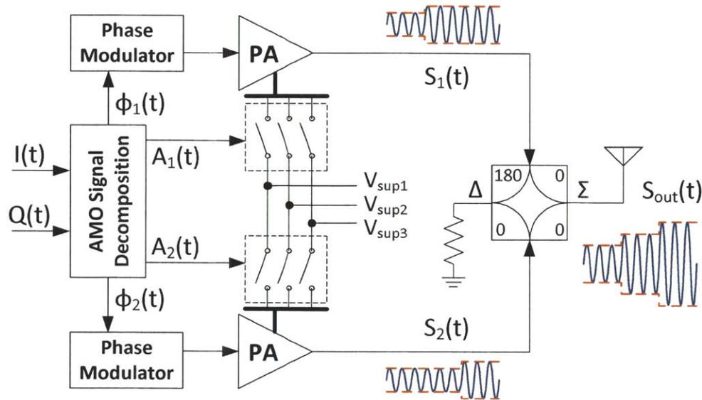
Figure 4-28: Asymmetric multilevel outphasing (AMO) transmitter with discrete supply-voltage modulation (DSVM). Three supply voltages are shown in the figure, but there can be any number of supply voltages greater than 1 for the AMO system.
