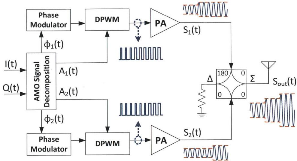
Figure 4-20: Asymmetric multilevel outphasing (AMO) transmitter with discrete pulse-width modulation (DPWM).
