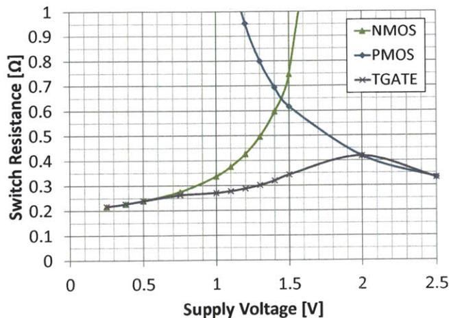
Figure 5-14: Power supply switch resistance vs. supply voltage when the switch is used to connect the PA supply voltage to the PA in the 2.4-GHz AMO IC prototype.
