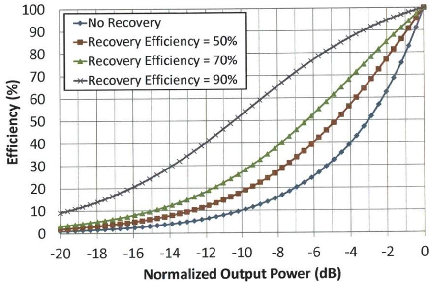
Figure 3-9: Theoretical OPERA efficiency as a function of normalized output power, showing the effect of the energy recovery network efficiency. The PAs are assumed to be 100% efficient, with no insertion loss in the power combiner.
