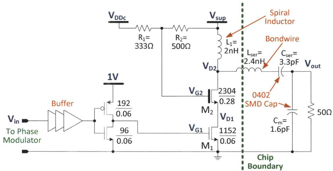
Figure 5-1: Circuit schematic of the class-E PA used in the 2.4-GHz AMO IC prototype. The single-ended version is shown for simplicity.
