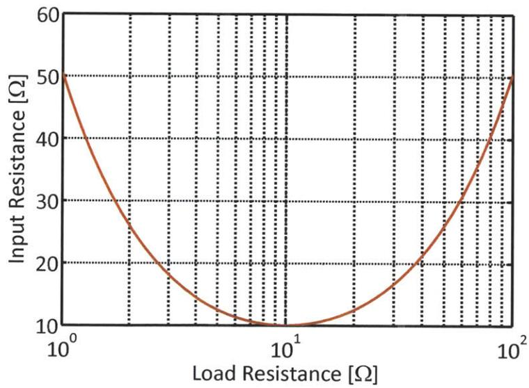
Figure 3-5: Input resistance  $R_{RCN}$  of the RCN shown in Figure 3-4 vs. load resistance  $R_{rect}$  for  $X = 10\Omega$ .
