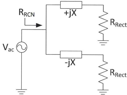
Figure 3-4: Two-element resistance compression network with reactive branches represented by impedances evaluated at the operating frequency.
