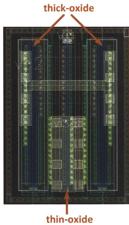
Figure 5-4: Layout view of a single unit cell for the cascode class-E PA in the 2.4-GHz AMO IC prototype.
