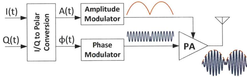
Figure 2-4: Conventional polar architecture.
