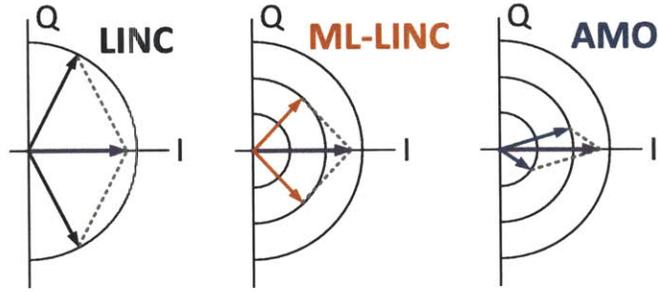
Figure 4-2: Signal component vector diagram for LINC, ML-LINC, and AMO. The smallest outphasing angle is achieved with AMO.
