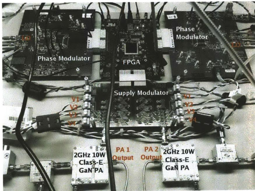
Figure 4-37: Prototype implementation of the 18-W 1.95-GHz AMO transmitter with discrete supply modulators and class-E GaN PAs. (a) block diagram, (b) photograph.
