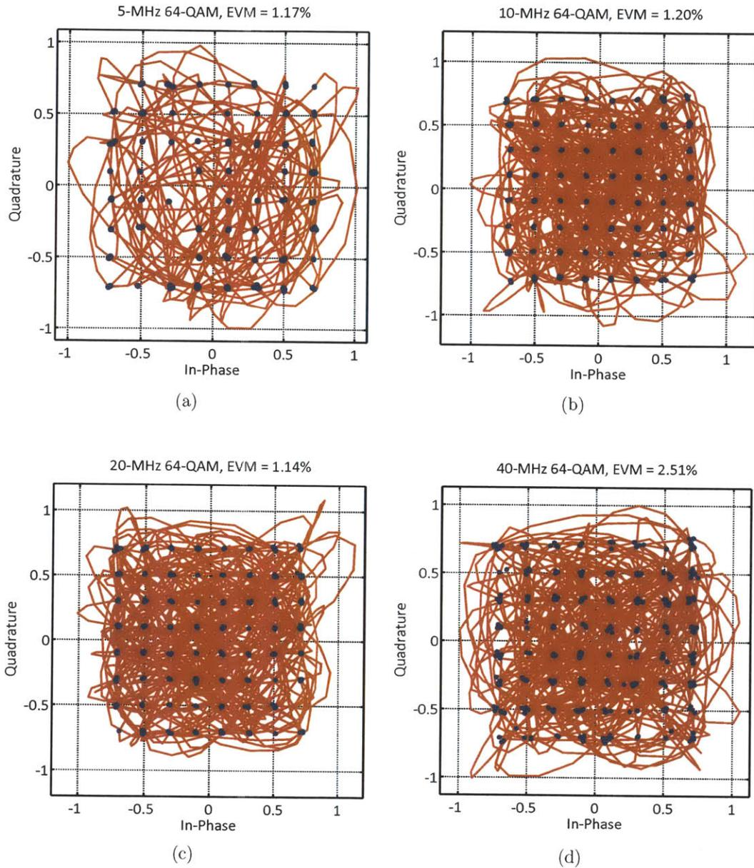
Figure 5-28: Constellation diagram of a 64-QAM signal transmitted by the AMO system at various symbol rates for the 2.4-GHz AMO transmitter. (a) 5 MHz. (b) 10 MHz. (c) 20 MHz. (d) 40 MHz.
