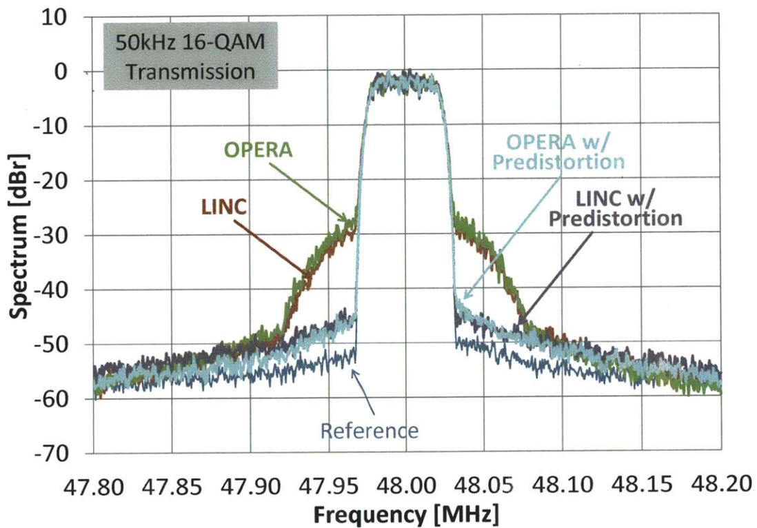
Figure 3-22: Measured output spectrum for 50-kHz 16-QAM transmission with 6.5-dB PAPR, with and without energy recovery, and before and after predistortion. The reference spectrum is the result using only the combiner with a fixed isolation port resistance.
