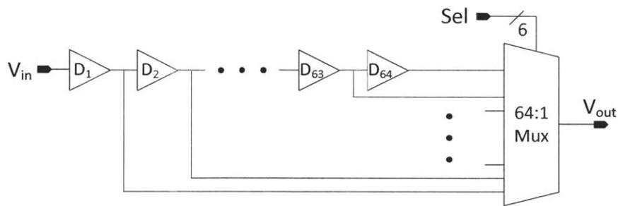
Figure 5-11: Block diagram of the delay line used in the delay adjustment circuit and to implement time alignment between the amplitude and phase paths for the 2.4-GHz AMO IC prototype.
