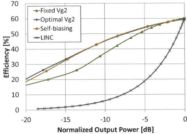
Figure 5-6: Simulated efficiency vs. output power of the cascode class-E PA in the 2.4-GHz AMO IC prototype, for different biasing schemes for the cascode device. The efficiency of the LINC system is also shown for reference.
