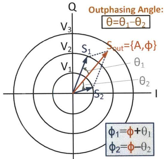
Figure 4-3: Vector diagram for AMO modulation, including notational convention.
