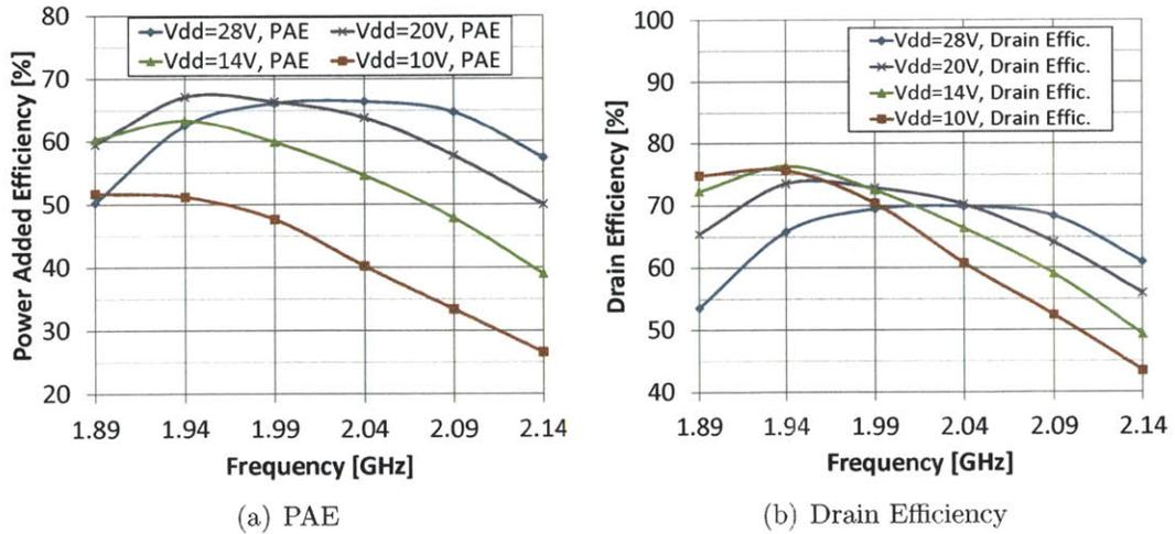
Figure 4-34: Measured PAE (a) and drain efficiency (b) vs. frequency at various supply voltages for the class-E GaN PA.
