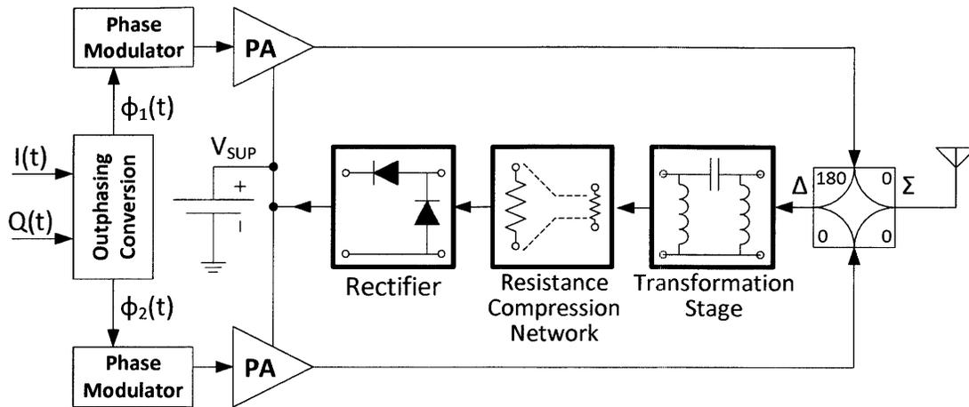
Figure 3-1: Outphasing energy recovery amplifier, utilizing a resistance compression network in the power recycling network.
