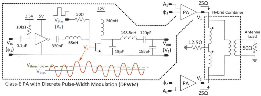
Figure 4-21: Prototype 48-MHz AMO transmitter with DPWM.
