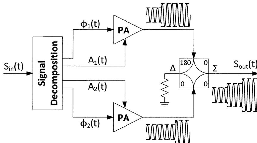
Figure 1-5: Asymmetric multilevel outphasing (AMO) architecture.
