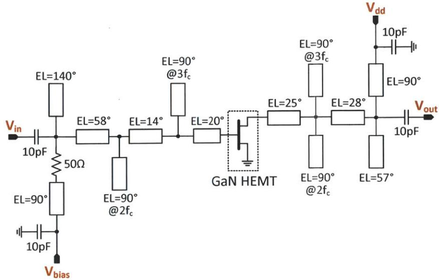
Figure 4-29: Circuit schematic of the 10-W class-E GaN PA. The design frequency was 2.14 GHz.  $EL$  stands for the electrical length of the given transmission line, and  $f_c$  stands for the RF carrier frequency.
