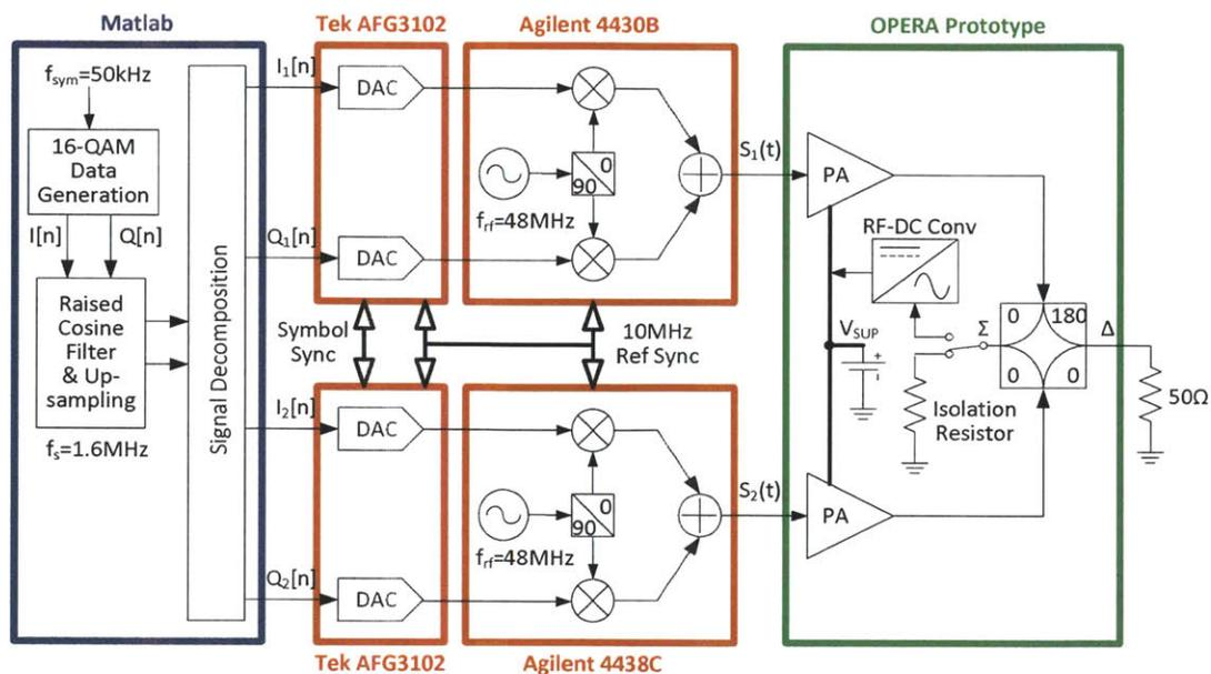
Figure 3-21: Outphasing system testbench used for the 48-MHz OPERA prototype for 50-kHz 16-QAM transmission.
