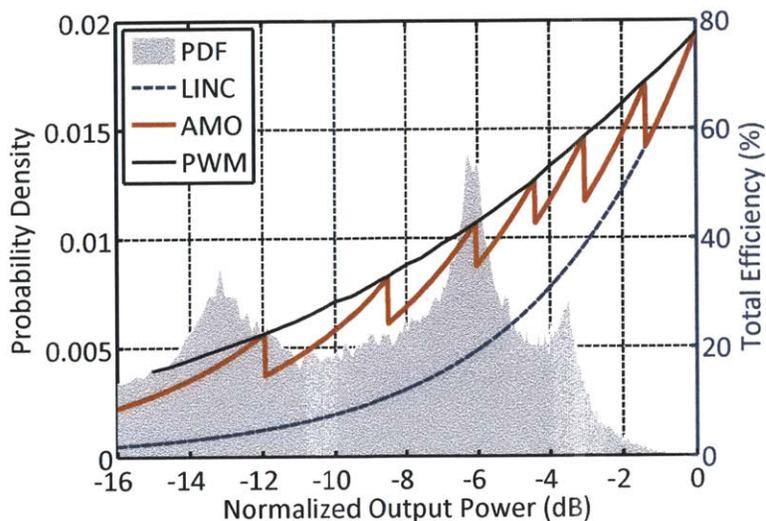
Figure 4-22: Measured PWM power-added efficiency vs. output power, along with the 4-level AMO efficiency optimized for a 16-QAM signal with 6.5-dB PAPR. The PDF of the 16-QAM signal is also shown.
