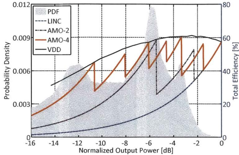
Figure 4-38: Measured efficiency vs. output power for the 1.95-GHz AMO prototype, along with the optimized amplitude levels for a 16-QAM signal with 6.5-dB PAPR. The PDF of the 16-QAM signal is also shown.
