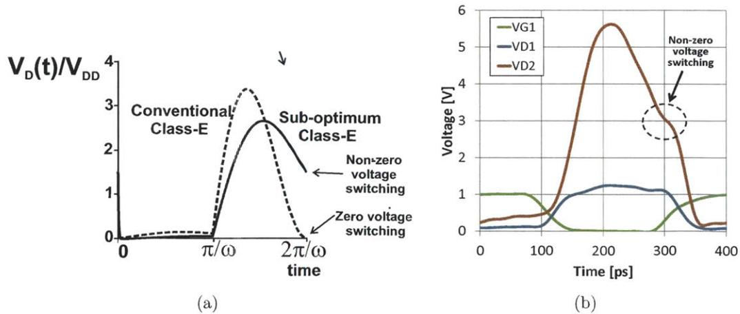
Figure 5-2: (a) Drain voltage waveforms for the conventional class-E PA and variable-voltage class-E PA. (b) Simulated drain voltage waveform for the PA used in the 2.4-GHz AMO IC prototype.
