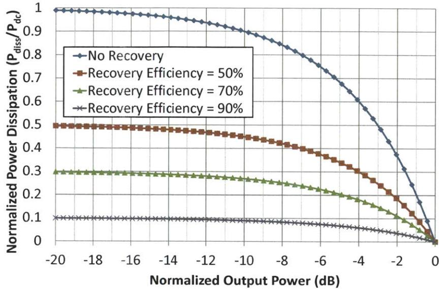
Figure 3-10: Theoretical OPERA power dissipation normalized to the total dc power sent to the PAs from the power supply, as a function of normalized output power, with the efficiency of the energy recovery network as a parameter. The PAs are assumed to be 100% efficient, with no insertion loss in the power combiner.
