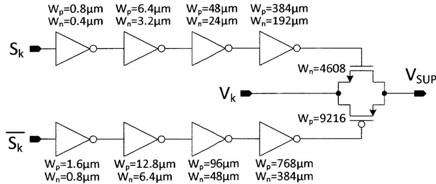
Figure 5-12: Transistor sizes for the power supply switches and the inverter chains used to drive them for the 2.4-GHz AMO IC prototype. The channel length of all the transistors is  $0.28 \mu\text{m}$ .
