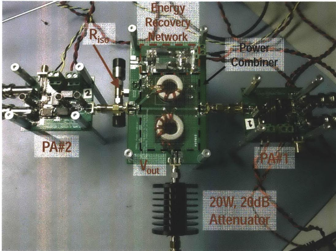
Figure 3-14: Photograph of the prototype OPERA system.
