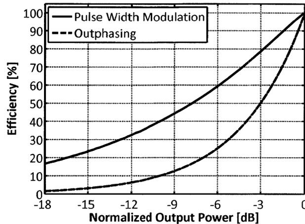
Figure 2-7: Comparison between the power efficiency of outphasing and pulse-width modulation depending on output power.
