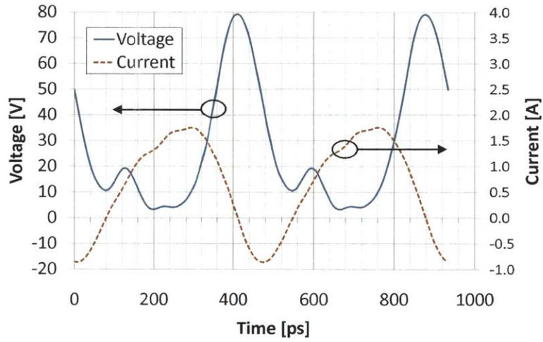
Figure 4-31: Simulated drain voltage and current for the class-E GaN PA after deembedding package parasitics, indicating class-E operation. The design frequency was 2.14 GHz.
