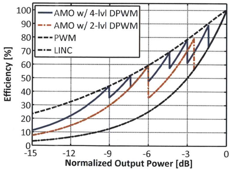
Figure 4-11: Efficiency for the AMO system using DPWM with 4 different duty cycles, along with the efficiency curve using 2 different duty cycles.
