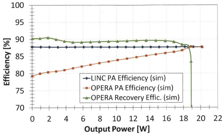
Figure 3-18: Simulated PA and power recycling efficiency for the OPERA prototype.
