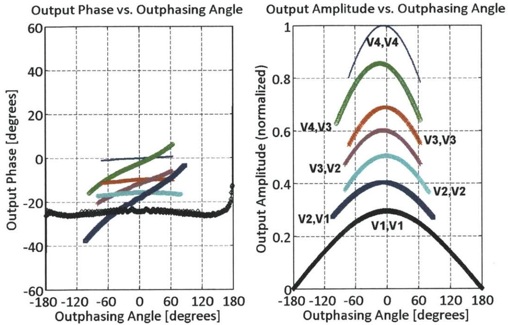
Figure 4-39: Measured static output amplitude and phase vs. outphasing angle for the 1.95-GHz AMO transmitter. Each curve corresponds to a different combination of supply voltages for the two outphased PAs.
