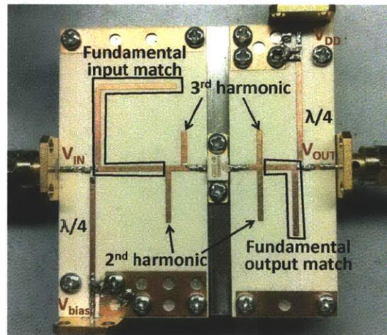
Figure 4-32: Photograph of the fabricated class-E GaN PA for the 1.95-GHz AMO prototype.
