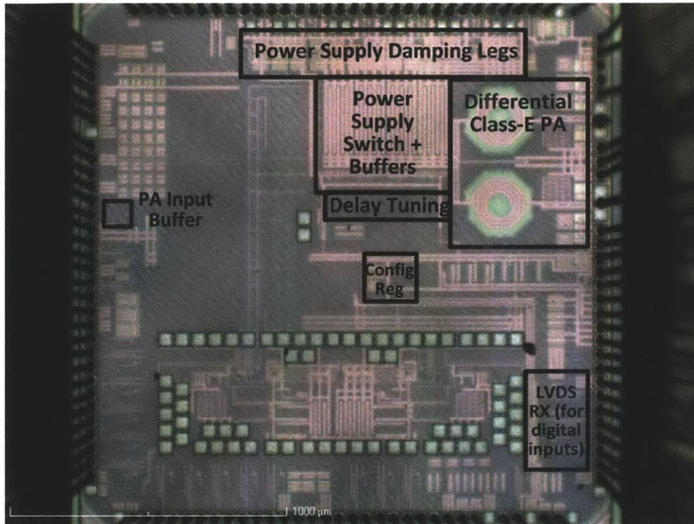
Figure 5-18: Die photo of the 2.4-GHz AMO IC prototype. The total chip area is  $2 \times 2 \text{ mm}^2$ . Each chip has one PA and one discrete supply voltage modulator.
