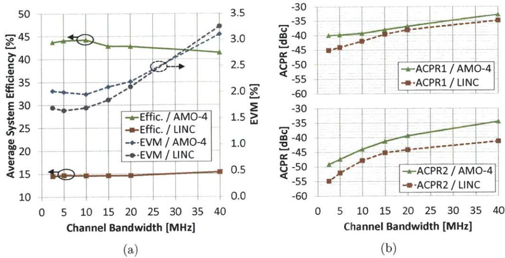
Figure 4-44: Performance comparison of the LINC and 4-level AMO systems for the 1.95-GHz AMO prototype, for the transmission of a 6.5-dB PAPR 16-QAM signal at various channel bandwidths. (a) EVM and average system efficiency. (b) ACPR at 1st and 2nd channel offsets.
