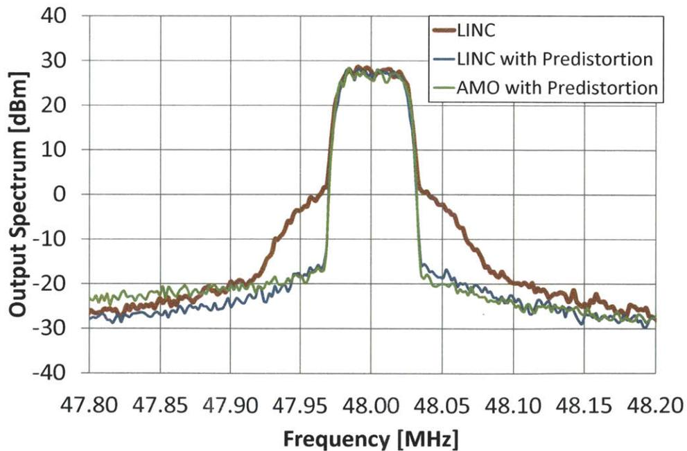
Figure 4-27: Measured transmit spectrum of the 50-kHz, 16-QAM signal for both the LINC and AMO-DPDM systems.
