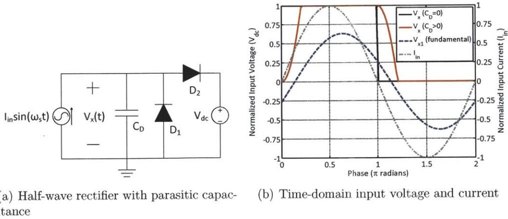
Figure 3-7: Half-wave rectifier with parasitic capacitance and driven by a sinusoidal current source, along with characteristic waveforms.
