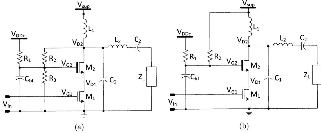
Figure 5-3: (a) Self-biasing topology for a cascode class-E PA used in [60, 61]. (b) Improved self-biasing topology used in this work.
