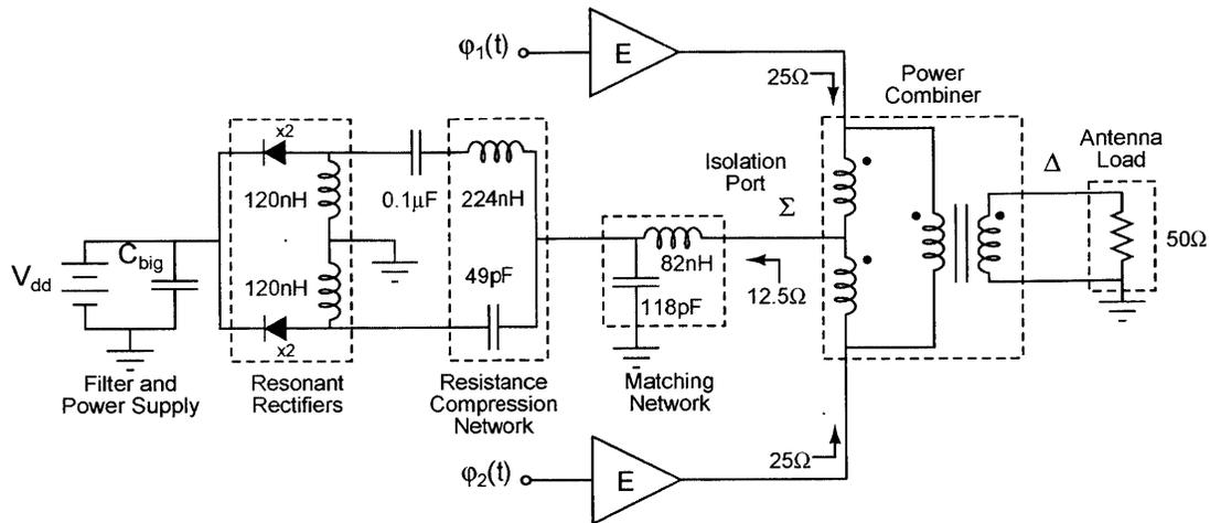
Figure 3-12: Prototype OPERA system with resistance-compressed rectifier for energy recovery. Each rectifier branch is implemented with a pair of paralleled SS16 Schottky diodes. The impedance at each port of the power combiner that is required for matching and isolation is also indicated.
