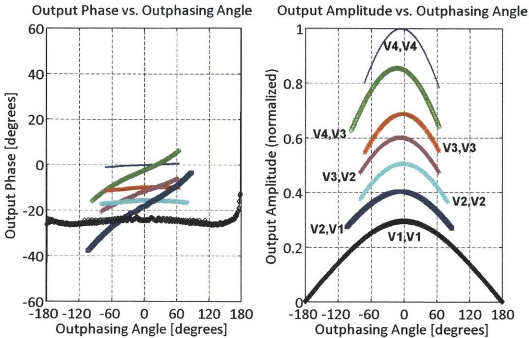
Figure 4-15: Example measurement data for the output amplitude and phase vs. outphasing angle for a real AMO system, which capture the static nonlinearities of the AMO system. Each curve corresponds to a different combination of amplitude levels for the two outphased PAs.
