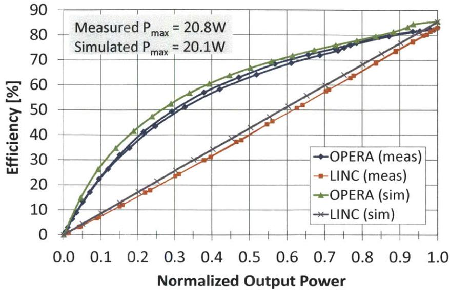
Figure 3-17: System efficiency vs. output power for the OPERA prototype.
