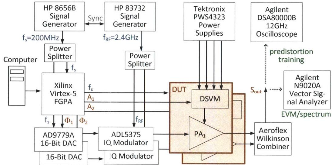
Figure 5-19: Testbench for the 2.4-GHz AMO IC prototype, composed of two CMOS class-E PAs and two discrete supply modulators.
