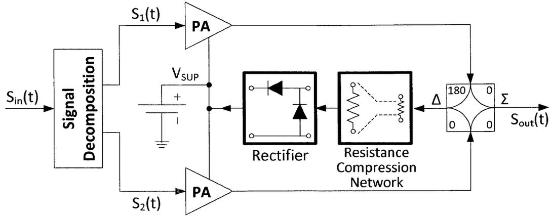
Figure 1-4: Outphasing energy recovery amplifier, utilizing a resistance compression network in the power recycling network.
