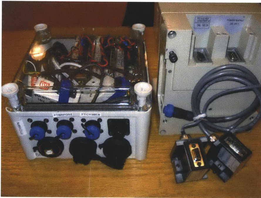
Figure B-6: Sensor support enclosure for three SICK laser scanners and one generic usb device to route through the internal USB hub.
