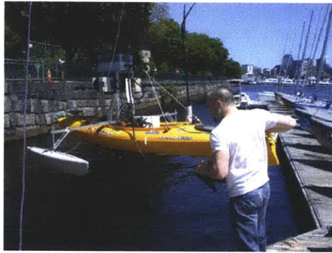
Figure 5-2: The small craft permits rapid vehicle launch and recovery with the aid of an electric hoist. Usually one operator performed the procedure, although we recommend two operators.
