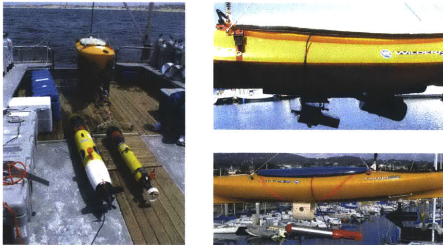
Figure 1-5: At left, two small autonomous underwater vehicles (AUVs) and a SCOUT autonomous surface craft (ASC) prior to deployment. A REMUS vehicle is shown to the left of the smaller lower cost iRobot Ranger. At right, simple mounting rigs enable the SCOUT autonomous surface craft (ASC) to rapidly deploy new sensors, such as a multiple imaging sonars (top) or a sidescan sonar (bottom).
