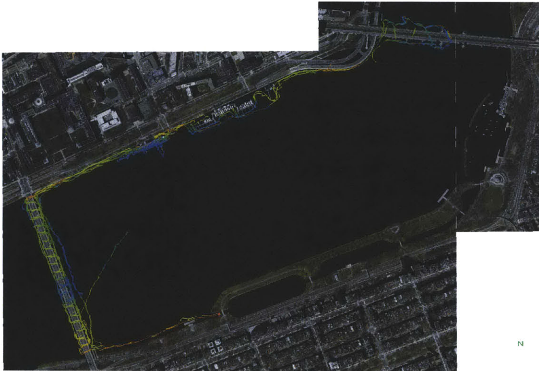
Figure 5-22: Bathymetry map created from fusing surface craft bathymetry submaps is overlaid on aerial imagery. Map is false colored with cooler colors (blue) deeper and warm colors (red) shallower. The limited sensor field of view and scale of the environment present significant challenges to achieving sensor coverage.
