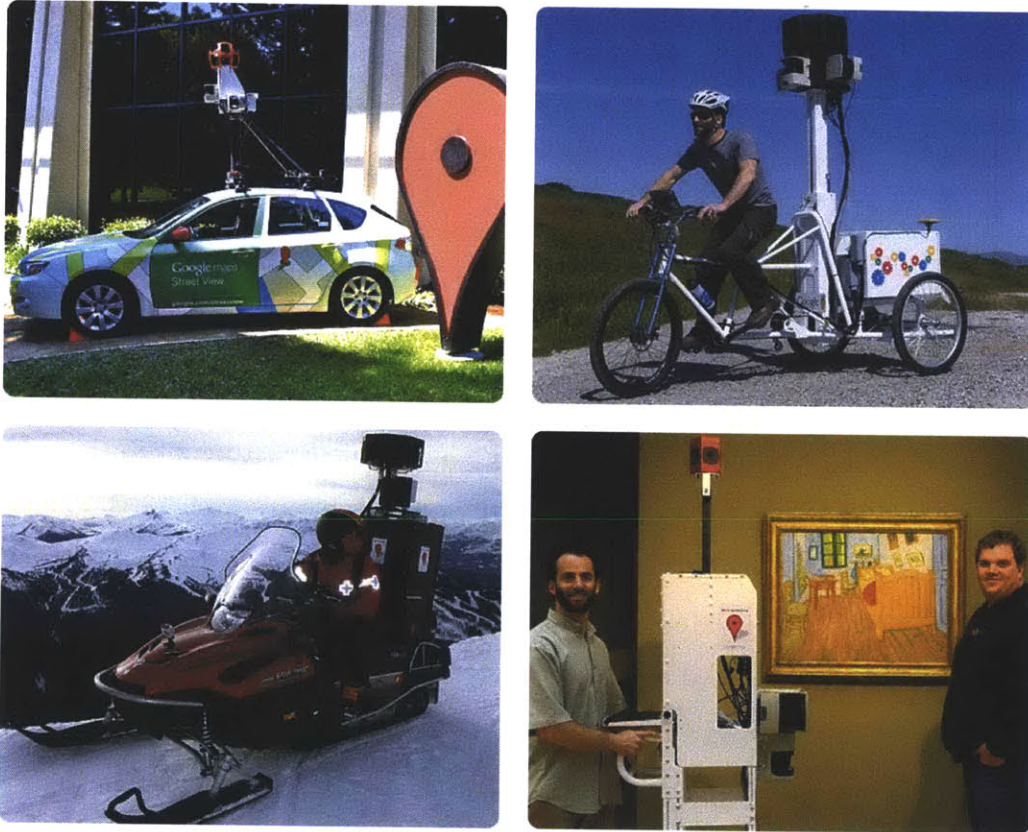
Figure 1-4: The Google Street View project employs a variety of platforms for capturing environments in 3D [67].
