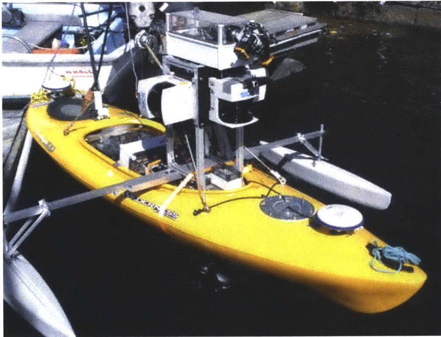
Figure B-1: The kayak and sensor suite is visible while being hoisted into the water.
