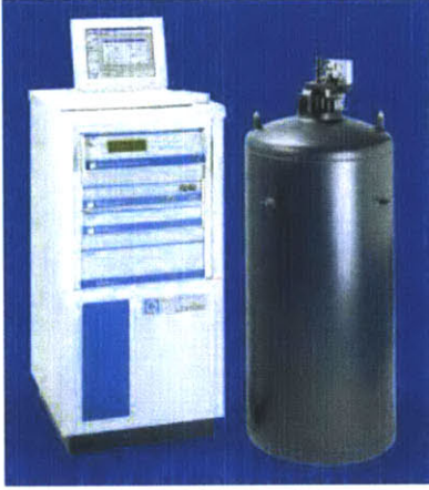
Figure 2-1: Photo of a Quantum Design (QD) Physical Property Measurement System (PPMS) apparatus. For the QD PPMS apparatus in Professor Opeil's laboratory at Boston College (BC), it has a temperature range of 2K to 400K and a magnetic field range of 0T to \pm 9 T. It has the capability to simultaneously measure the \kappa_{th} , S , and \rho , as well as the R_H .
