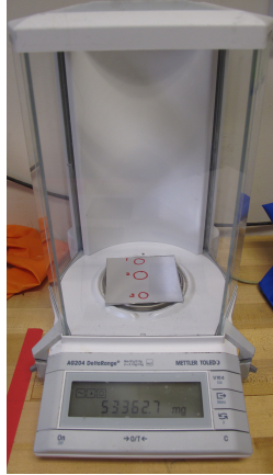
Figure 6-6: Mass measurement with Mettler Toledo Balance
