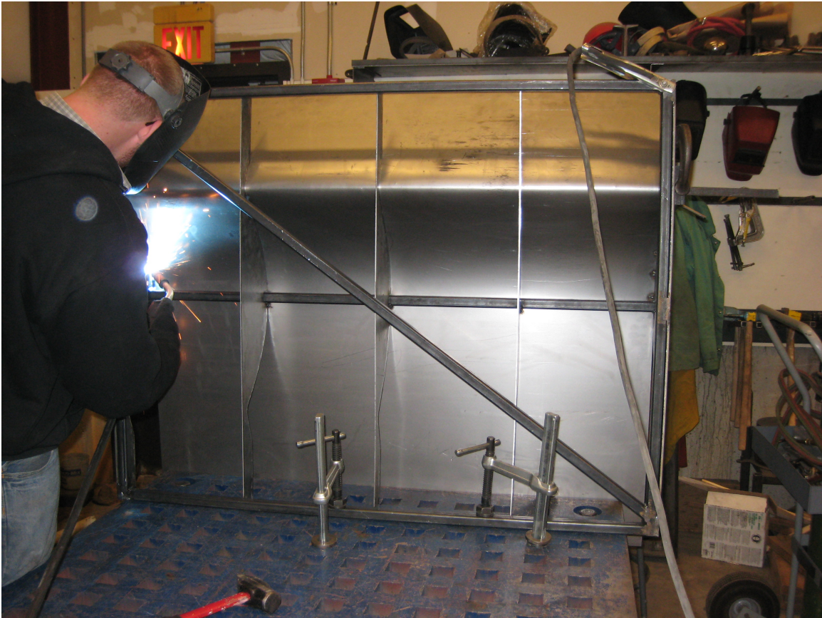
Figure A-3: Welding skin onto steel frame
