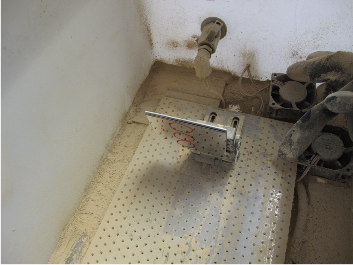
Figure 6-11: Inside dust chamber with mirror film sample
