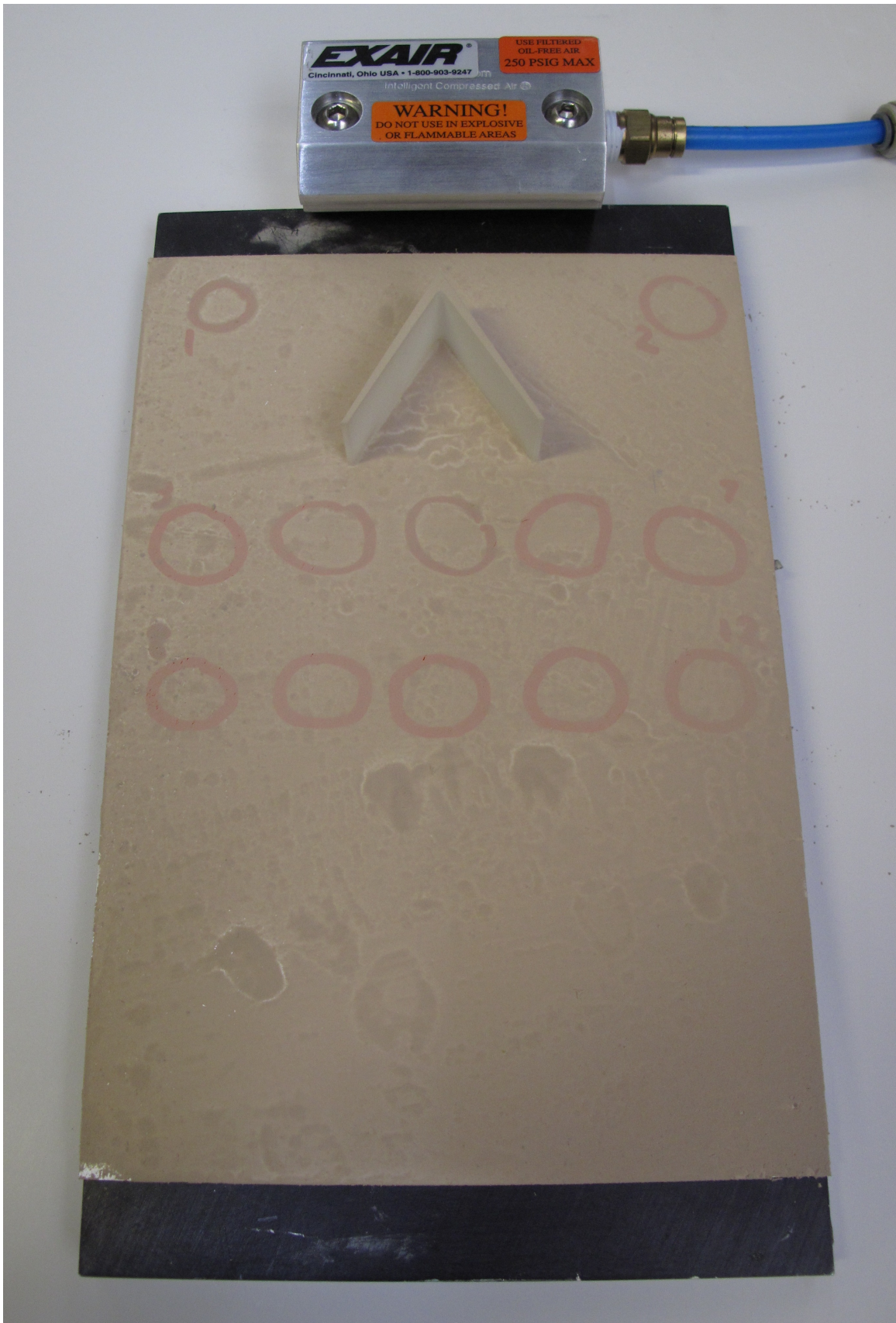
Figure 7-17: Vortex generator on mirror film surface after 23 minute contamination in dust chamber.
