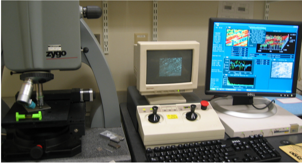
Figure 5-1: Zygo optical surface profilometer for surface roughness measurements.
