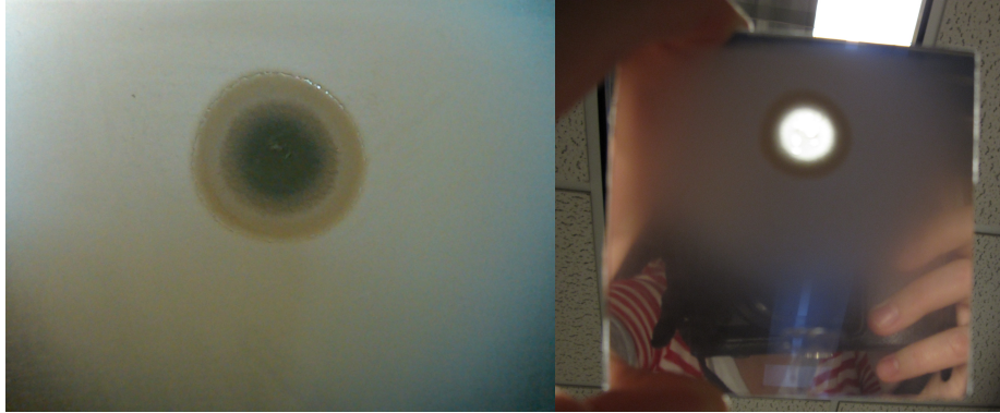
Figure 5-7: Mirror film sample after exposure to quartz directed quartz particle erosion with front-lit surface (left) and back-lit image of same sample (right).
