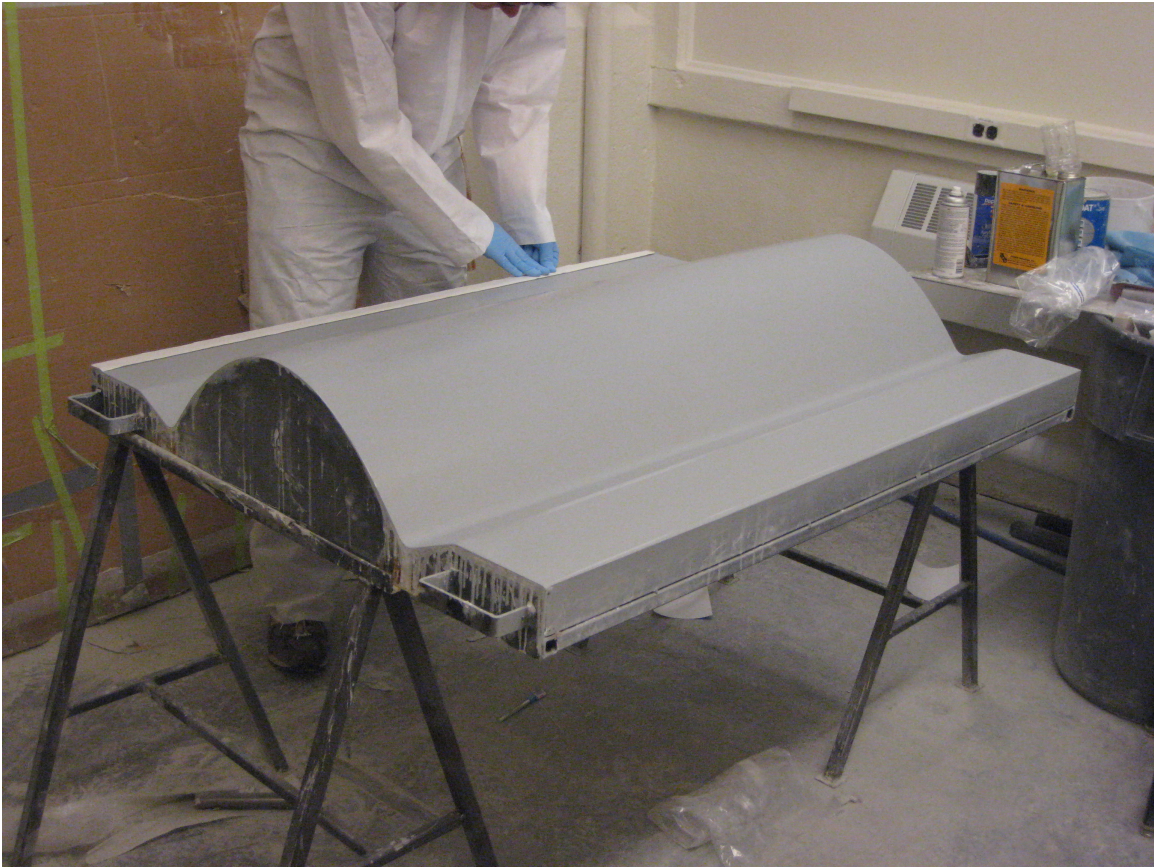
Figure A-6: Final mold surface after filler smoothing.
