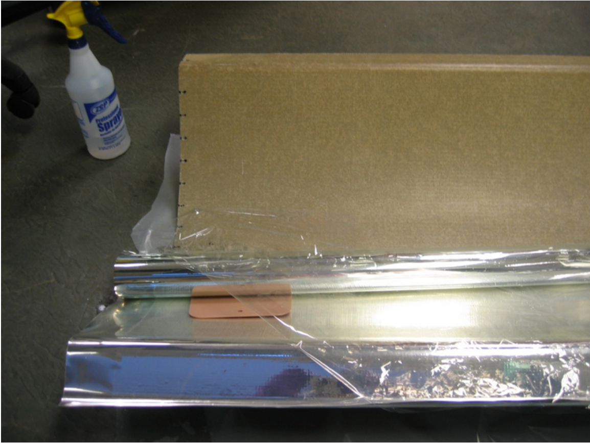
Figure B-4: Mirror film application with half of the film applied to the fiberglass part.
