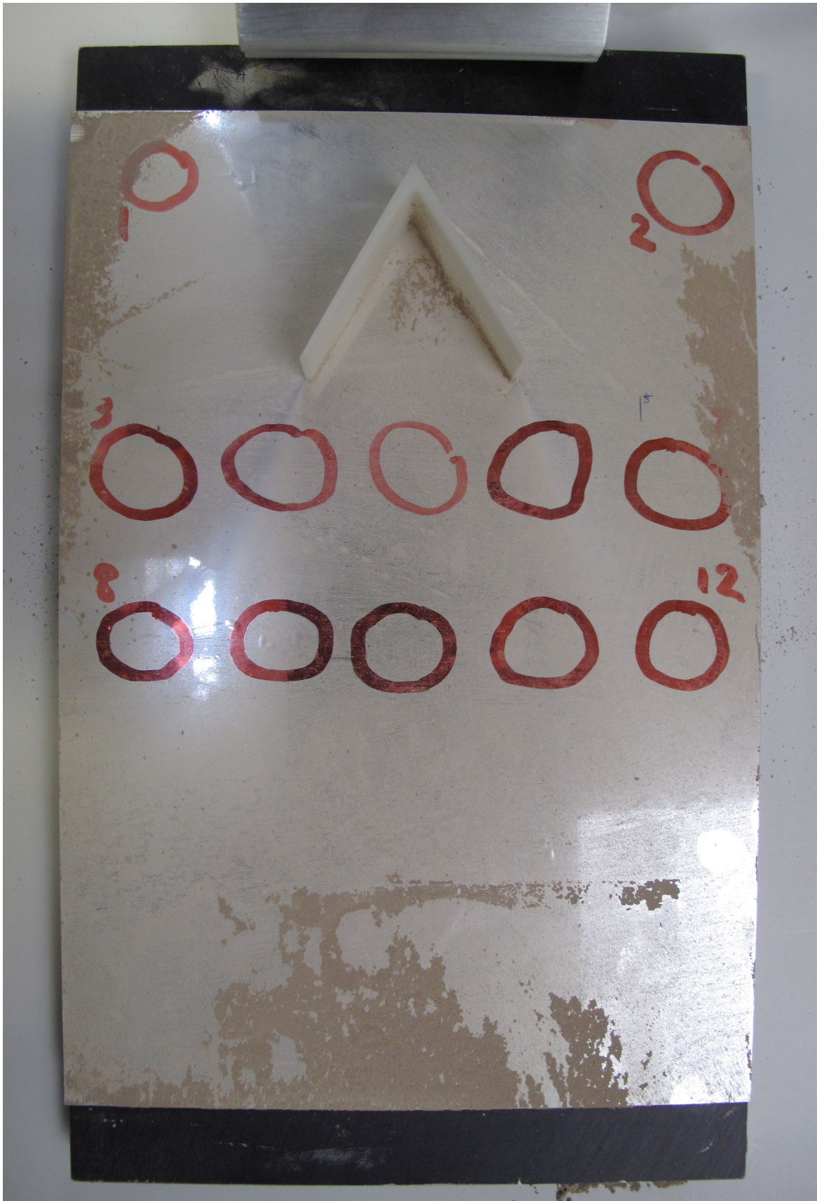
Figure 7-18: Vortex generator on mirror film surface after 5.9m/s airflow over panel.
