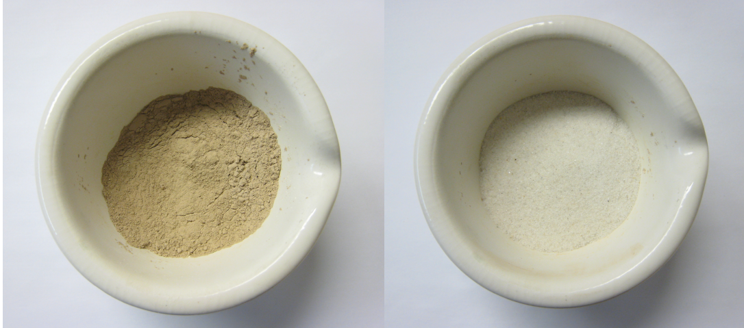
Figure 6-1: Arizona Medium Test Dust (left) and Mil Quartz (right).
