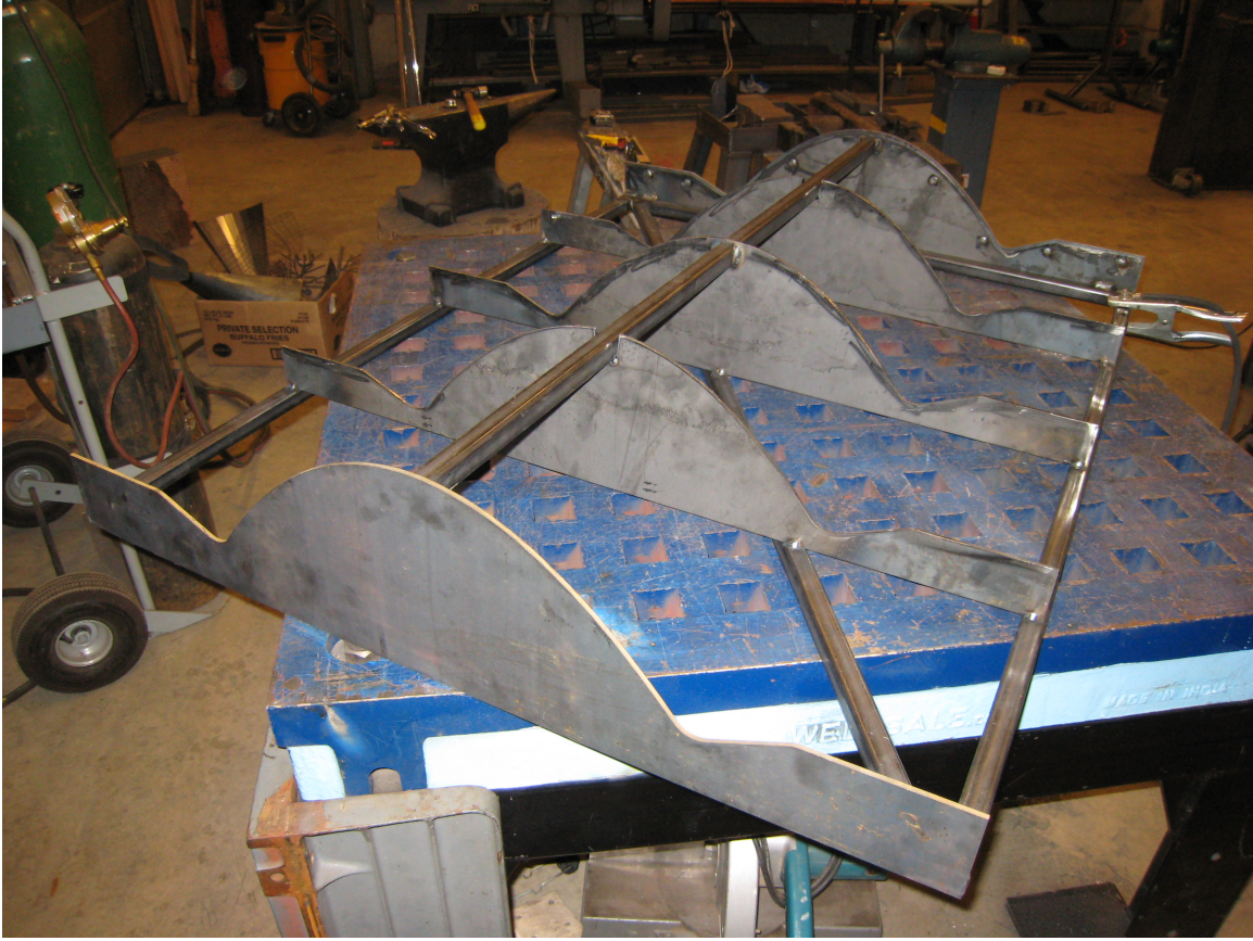
Figure A-2: Framing of Parabolic Trough Mold
