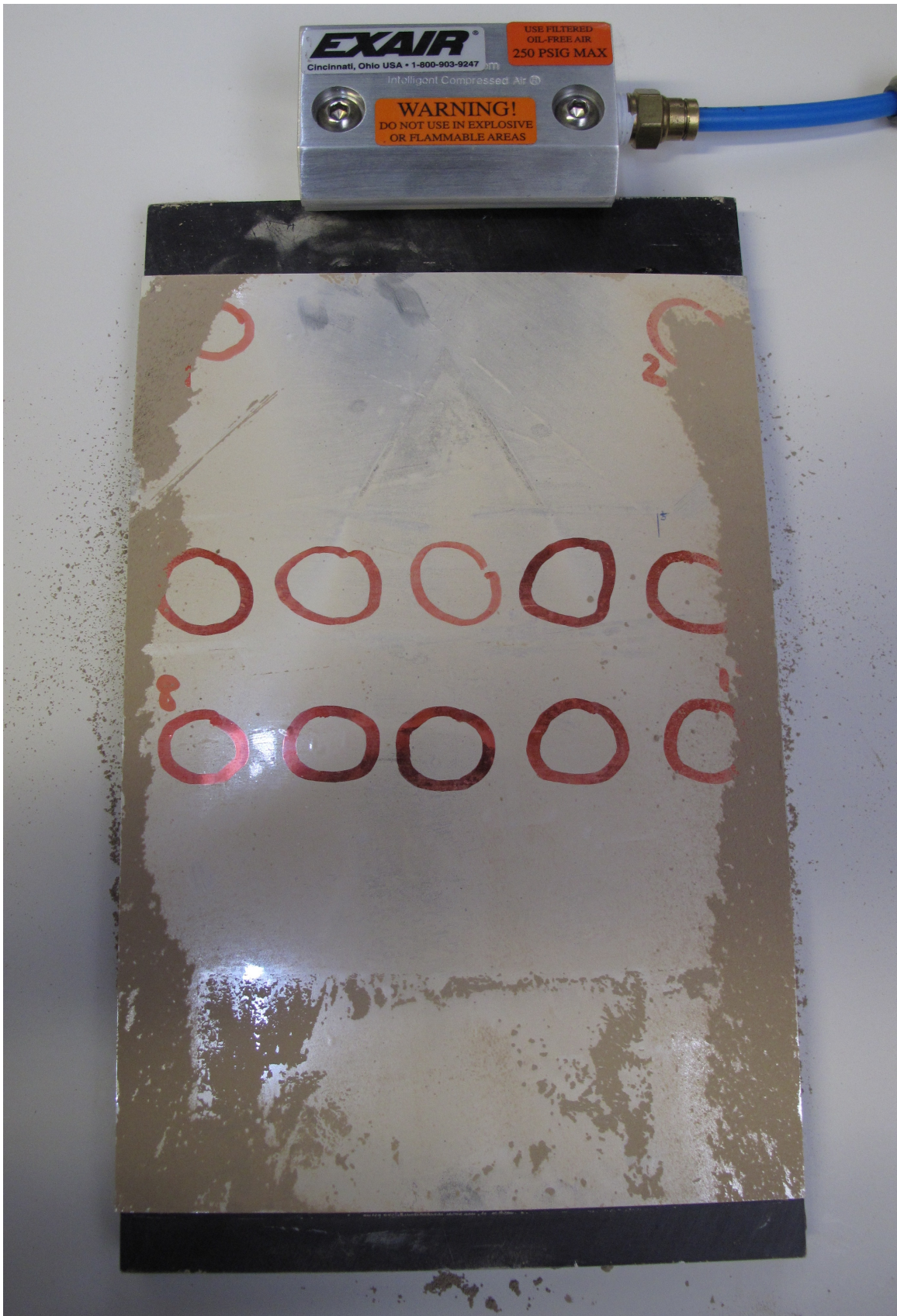
Figure 7-20: Mirror film surface after 5.9m/s airflow over panel with vortex generator absent.
