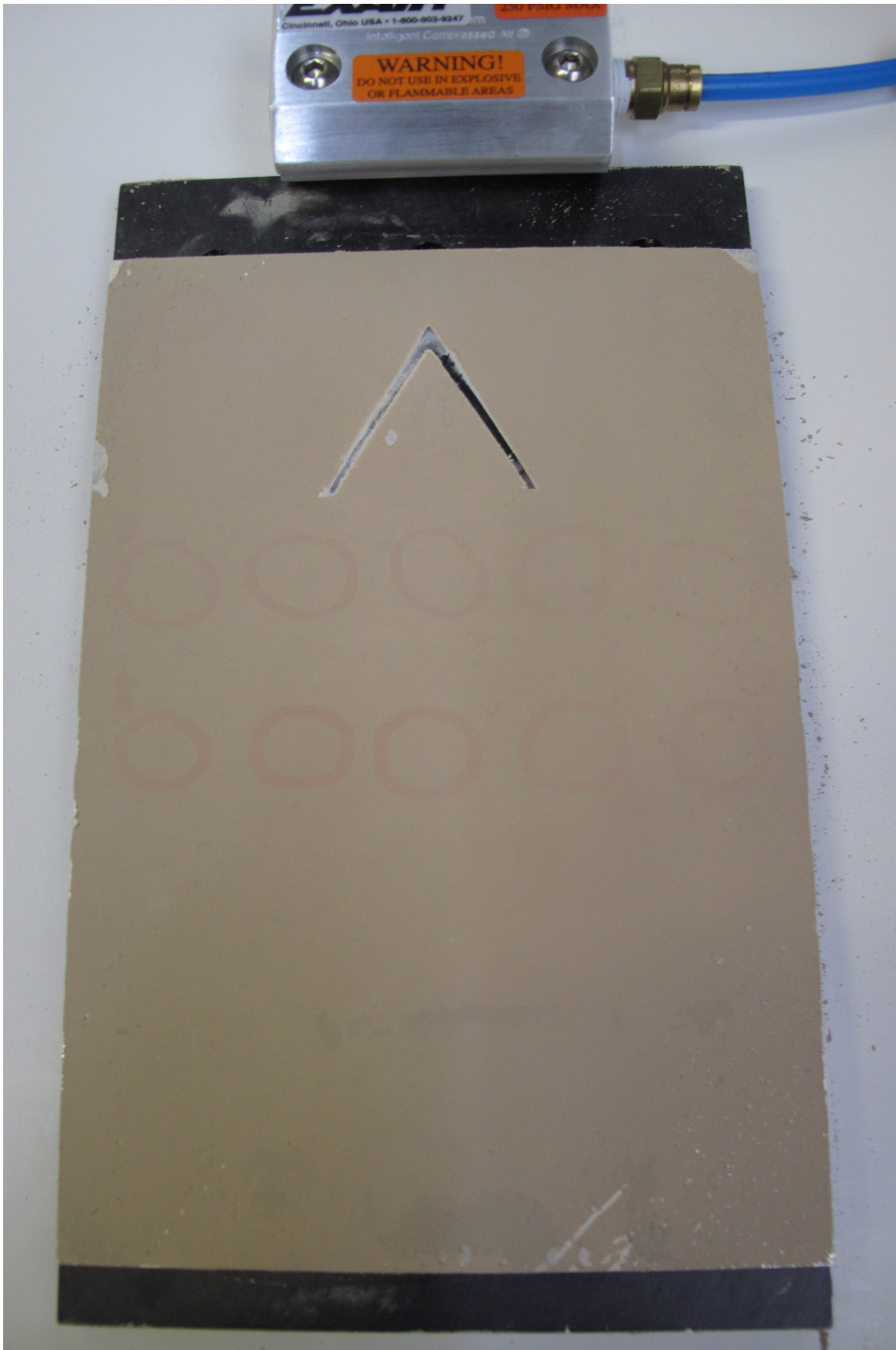
Figure 7-19: Mirror film surface after 23 minutes of contamination in dust chamber with previous vortex generator location shown.
