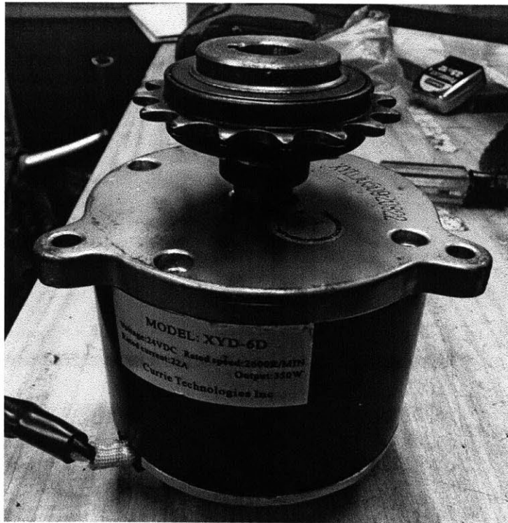
Fig. 4-3. Motor, with sprocket welded on collar on the shaft for the chain drive.
