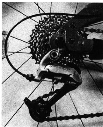
Fig. 2-4. Derailleur shifting mechanism on a modern bicycle (Photo credit: http://tinyurl.com/derailleur-source )
