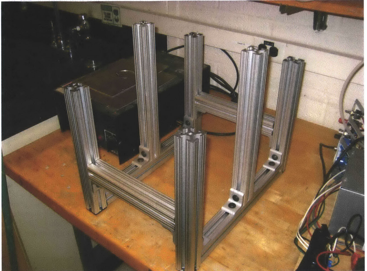
Figure 3: Example of the 80/20 Aluminum frame used to house the thermal system.
