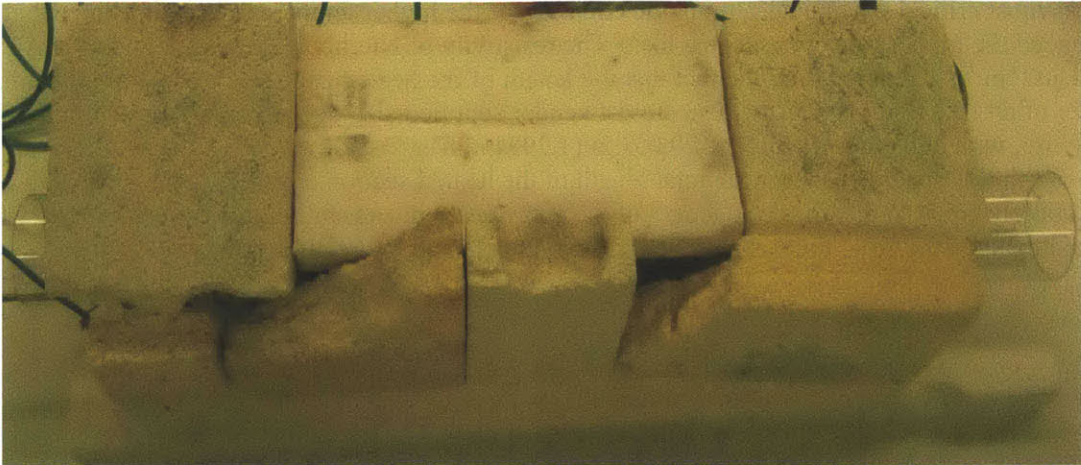
Figure 9: Insulation blocks placed around the quartz tube to provide a quick-and-dirty test of the nichrome wire.
