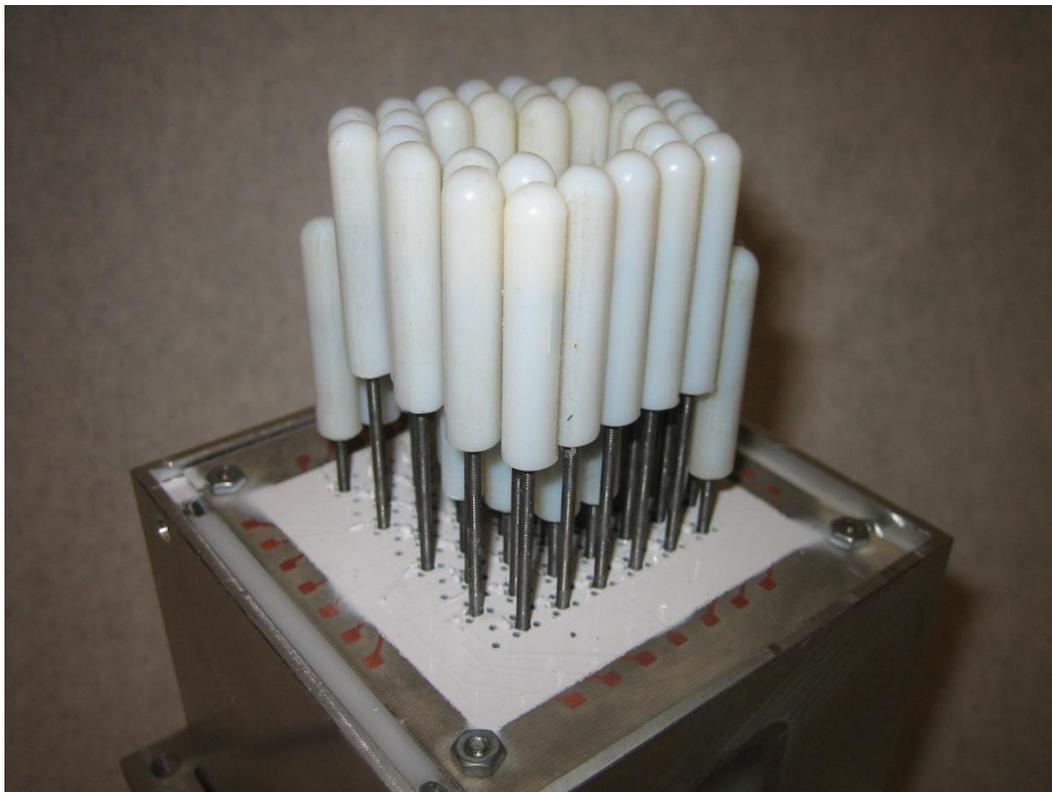
**Figure 1: Completed 52 pin, 0.3" pin spacing prototype; array size is 2" by 2".**
