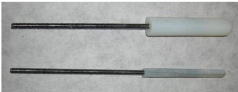
**Figure 18: A low resolution pin, 0.3" diameter (top) and a higher resolution pin 0.15" diameter (bottom).**
