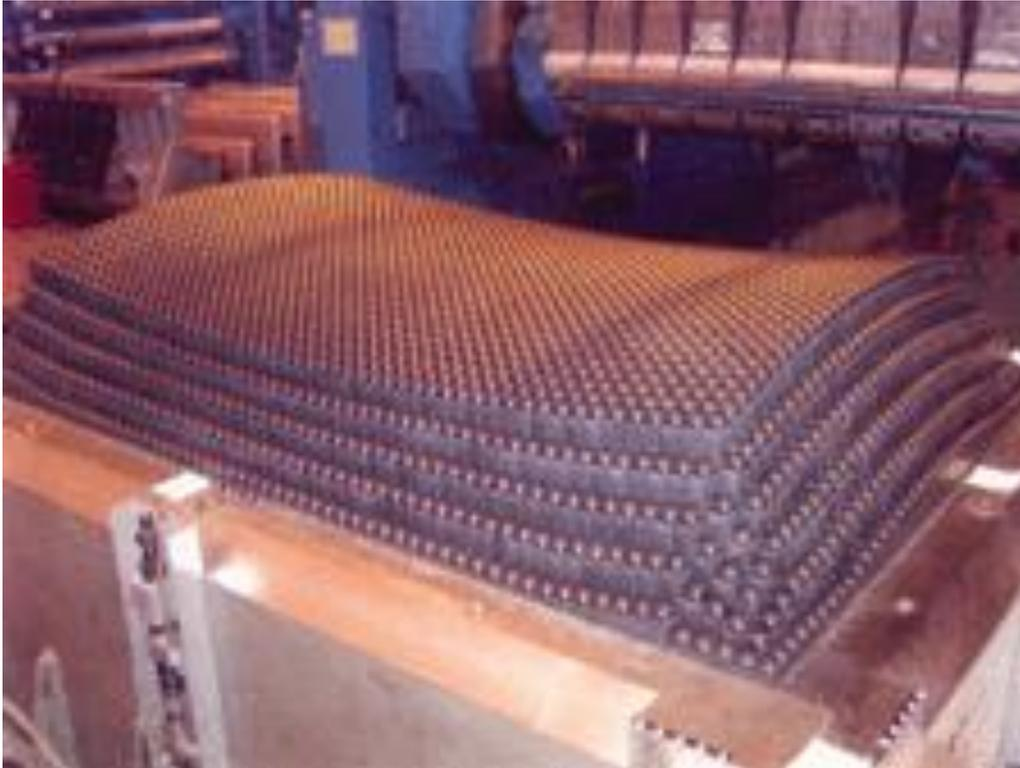
**Figure 2: Hardt's reconfigurable sheet metal forming die; composed of over 2,500, 1.125 inch square pins. Used modular DC motor and leadscrew pin actuation [2].**
