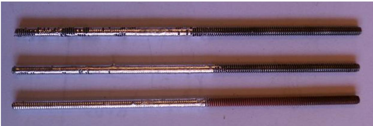
**Figure 19: Solder wetting of (top) oily threaded rod, (middle) clean rod, and (bottom) copper plated rod.**
