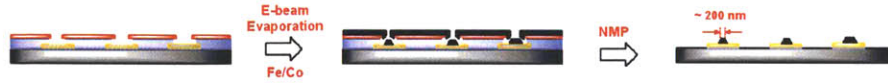
Figure 3.1: Our previous method for fabricating nanomagnets (Developed by Ben Chui at Stanford). The method is based on evaporation of Fe and Co through small holes, defined by E-beam lithography, into a cavity underneath the mask. The magnets are exposed by N-methylpyrrolidone (NMP) liftoff.
