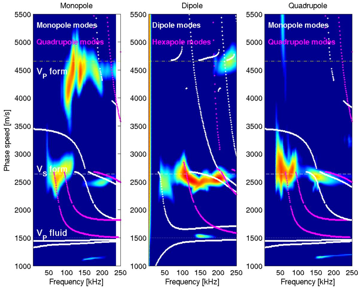
Figure 10: Sandstone borehole, source and receiver sections separated: Dispersion analysis results
