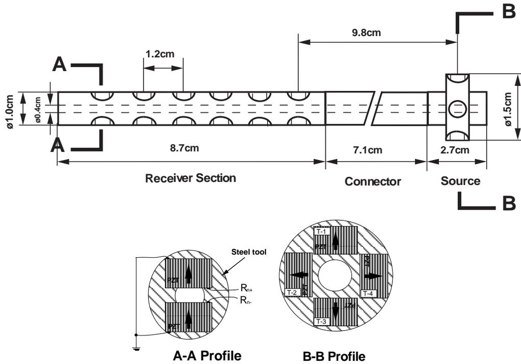
Figure 1: Schematic diagram of a scaled multipole logging tool with a source and six receiver pairs. The single transducer is a PZT cylinder crystal with 0.64 cm in diameter and 0.37 cm in thickness. The arrows indicate the polarization of the piezoelectric crystal.
