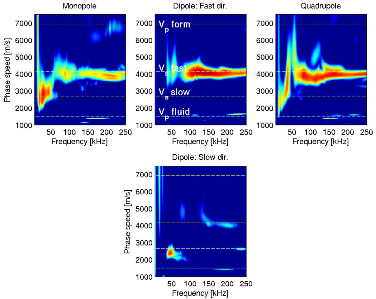
Figure 13: Slate borehole, source and receiver sections separated: Dispersion analysis results
