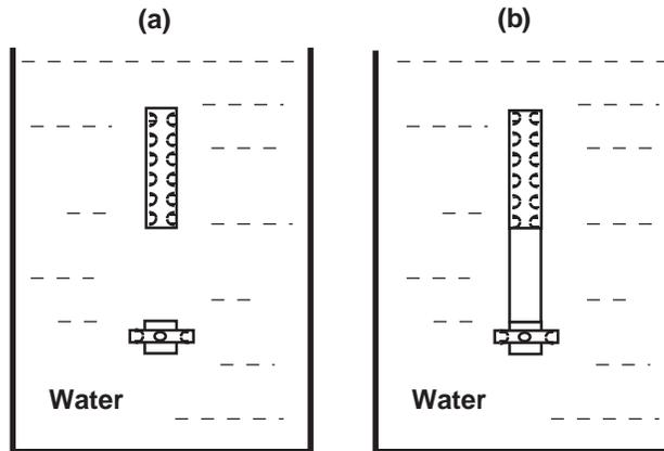
Figure 4: Schematic diagram of the measurements in a water tank without (a) or with (b) the connector.
