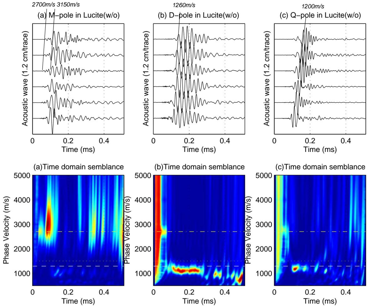
Figure 7: Lucite borehole, source and receiver sections separated: Acoustic waveforms and their semblance plots in time domain when the multipole tool works in the Lucite borehole at monopole (a), dipole (b), and quadrupole (c) modes. The center frequency of the electric signal exciting the source is 50kHz. The dash line indicates the P-wave and S-wave velocities in Lucite, and P wave velocity in water. A plastic centralizer is used to maintain the tool in the center of the borehole.
