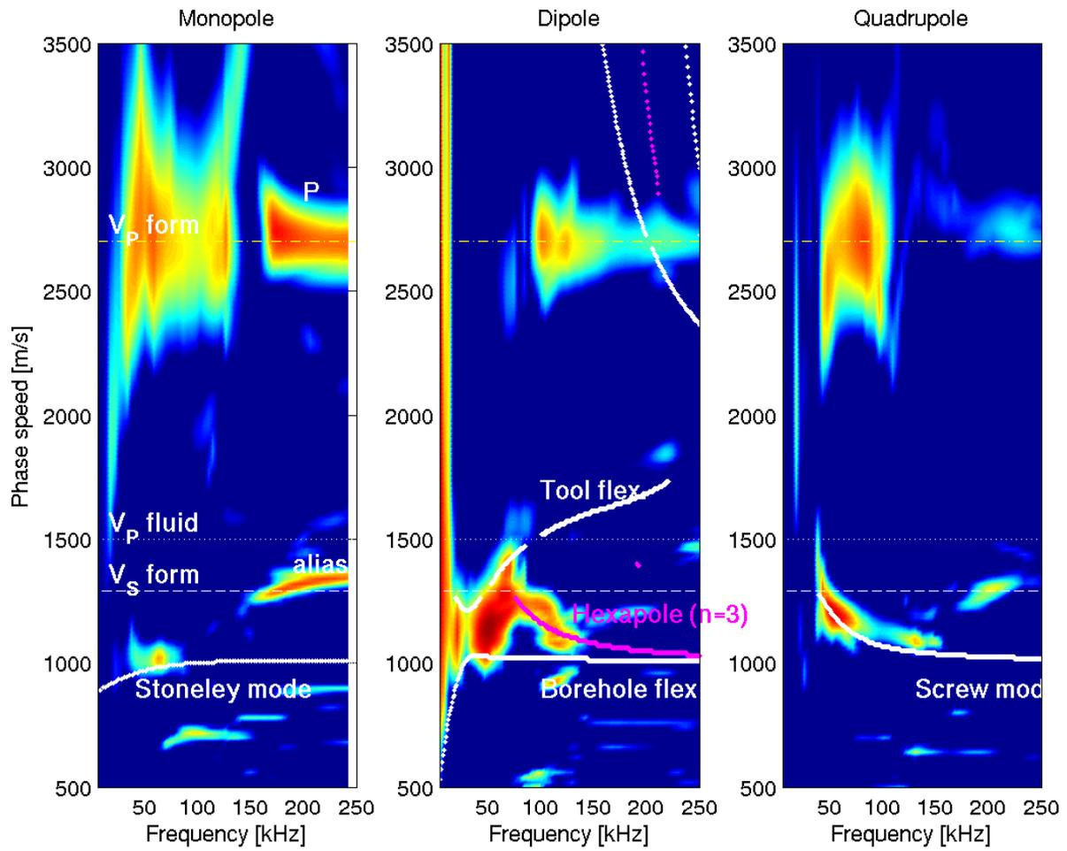
Figure 8: Lucite borehole, source and receiver sections separated: Dispersion analysis results
