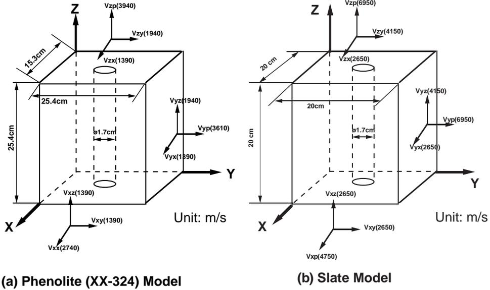
Figure 3: Distribution of the velocities in Phenolite XX-324 (a) and slate (b). Both are transverse isotropic in X direction and anisotropic in Z direction. The slow shear velocity in Phenolite is slower than water (1480m/s).
