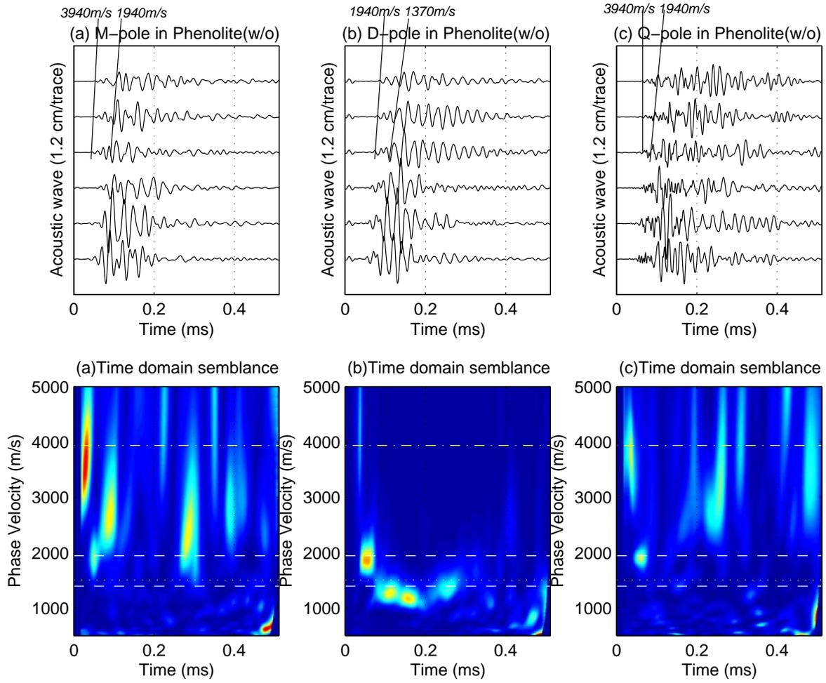
Figure 11: Phenolite borehole, source and receiver sections separated: Acoustic waveforms and their semblance plots in time domain when the multipole tool works in the Phenolite borehole at monopole (a), dipole (b), and quadrupole (c) modes. The center frequency of the source electric signal is 50kHz.
