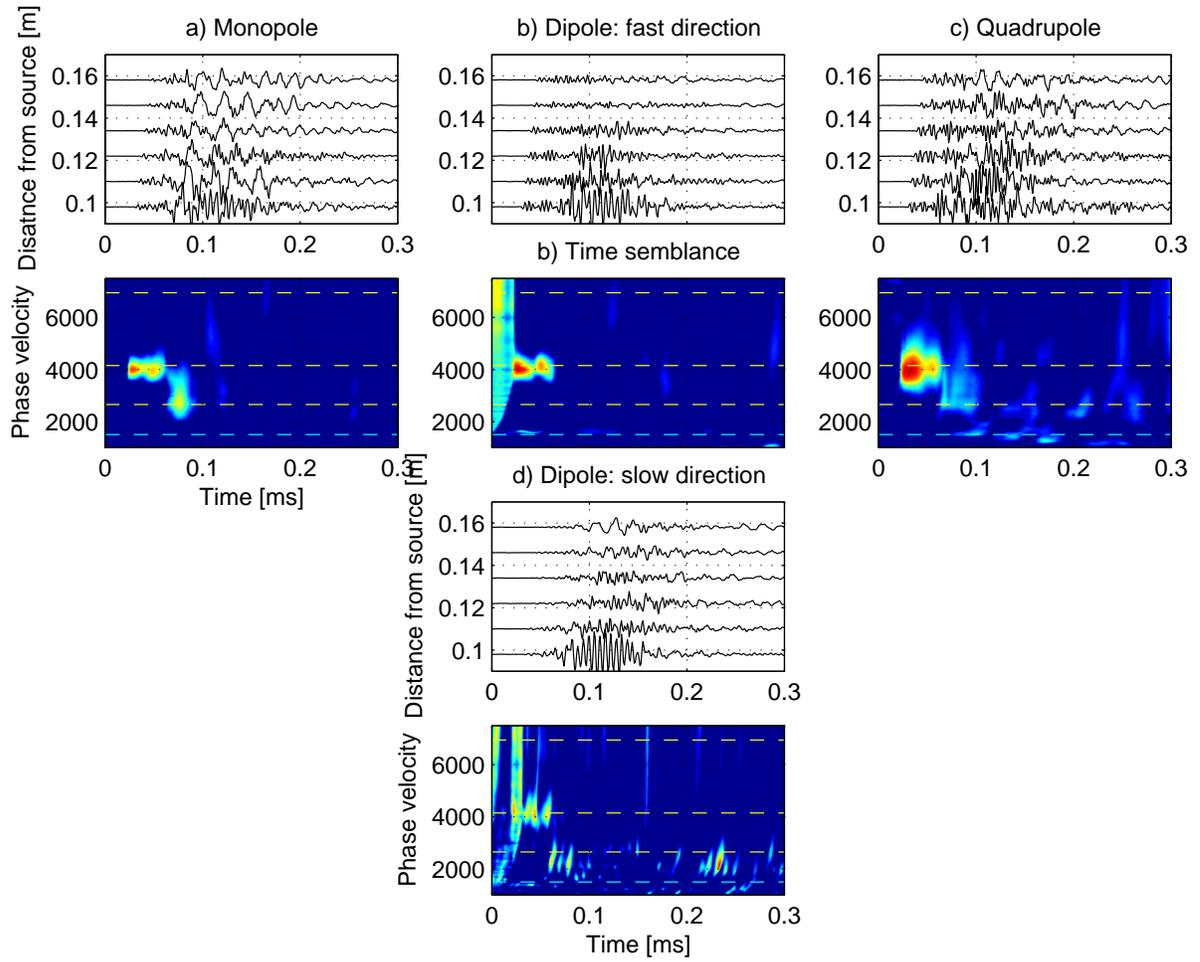
Figure 12: Slate borehole, source and receiver sections separated: Acoustic waveforms and their semblance plots in time domain when the multipole tool works in the slate borehole at monopole (a), dipole (b), and quadrupole (c) modes. The center frequency of the source electric signal is 50kHz.
