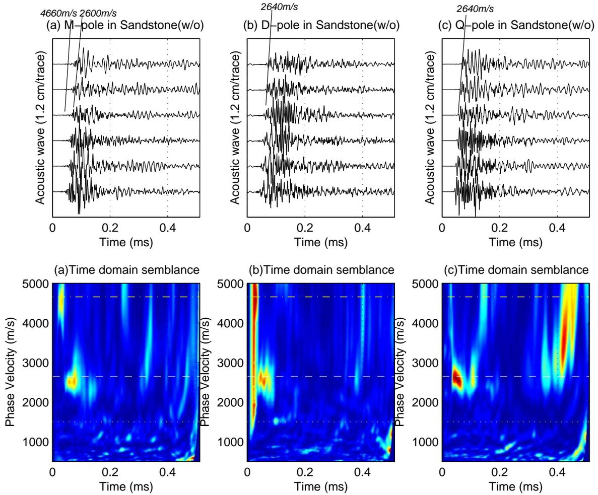
Figure 9: Sandstone borehole, source and receiver sections separated: Acoustic waveforms and their semblance plots in time domain when the multipole tool works in the sandstone borehole model at monopole (a), dipole (b), and quadrupole (c) modes without the connector. The center frequency of the source electric signal is 50kHz.
