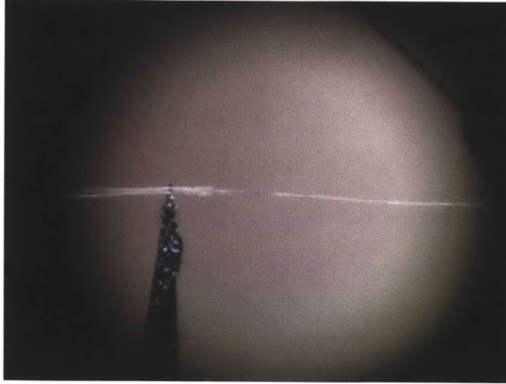
Figure 4-1: Polymer fiber with heating tungsten needle in contact near the polymer droplet end under optical microscope at 90X magnification. It is being heated in order to cut it where the fiber is thick and obtain the thinner sections of the fiber for storage.
