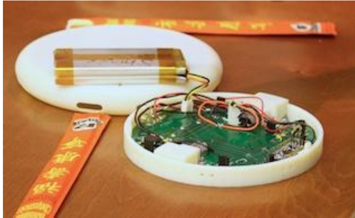
Figure 4-9: SushiBot technical review prototype – autonomously controlled by an Arduino microcontroller and IR sensors through line following navigation. SushiBot has a 3D printed chassis, a custom PCB, and plate detection capability with several response dances.
