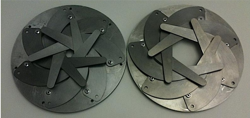
Figure 4-4: Tourné-Do Iris sketch model prototype - a seven blade iris diaphragm tourné cutting mechanism.
