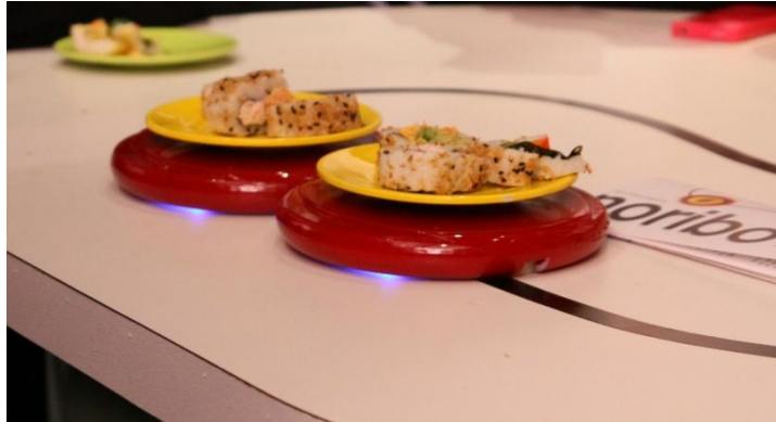
Figure 4-10: Noribo final presentation prototype – the next generation of SushiBot from the technical review. Noribo was manufactured in the same way and with the same components as its predecessor, but hardware and aesthetic improvements were made.
