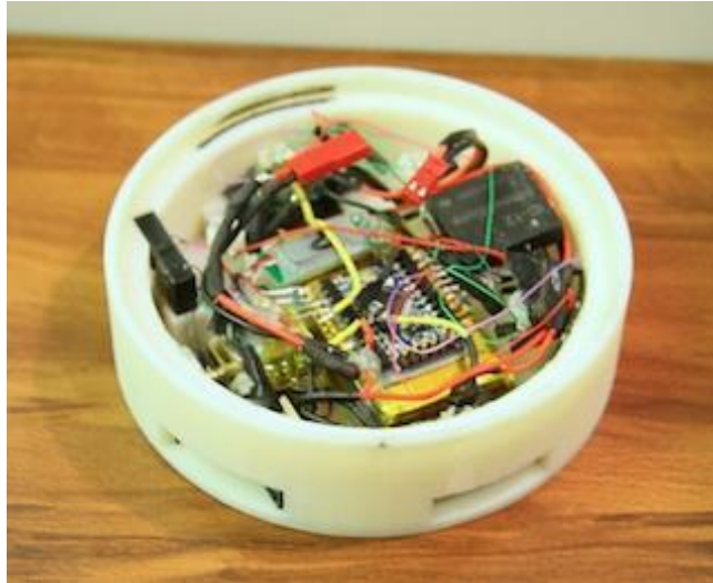
Figure 4-8: CoasterBot mock-up prototype – autonomously controlled by an Arduino microcontroller and IR sensors through wall following navigation. The chassis is 3D printed instead of laser cut.
