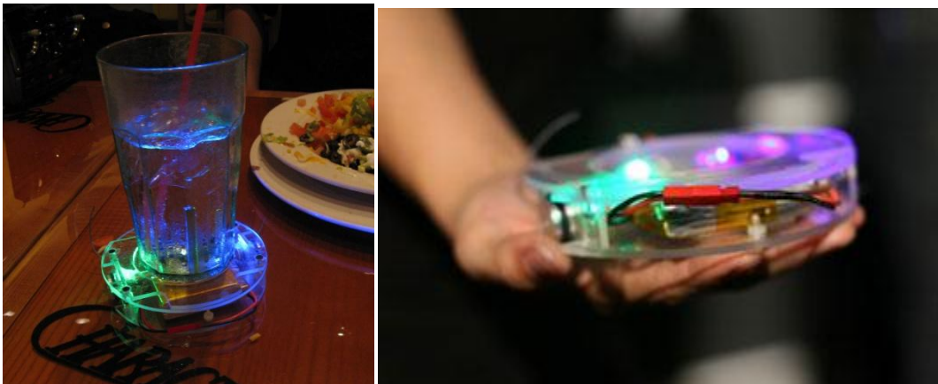
Figure 4-6: CoasterBot sketch model prototype - a remote controlled coaster shaped robot for delivering drinks to patrons at a bar. It is laser cut out of acrylic.
