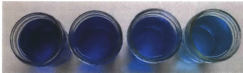
Figure 21: Glasses containing water dispensed by the prototype. Glasses contain (from left to right) simulated Whole, 2%, 1% and Skim
