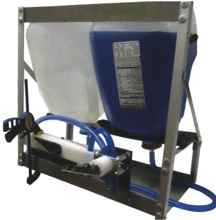
Figure 19: Picture of the final prototype. The tanks contain colored and clear water for observing mixing
