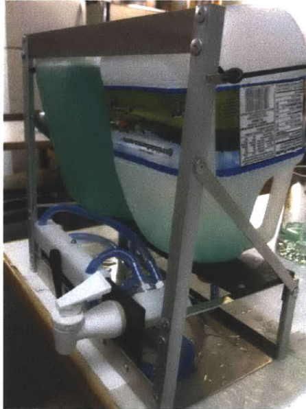
Figure 17: First full assembly of the milk machine. Notice the backflow of the colored water into the clear water tank.
