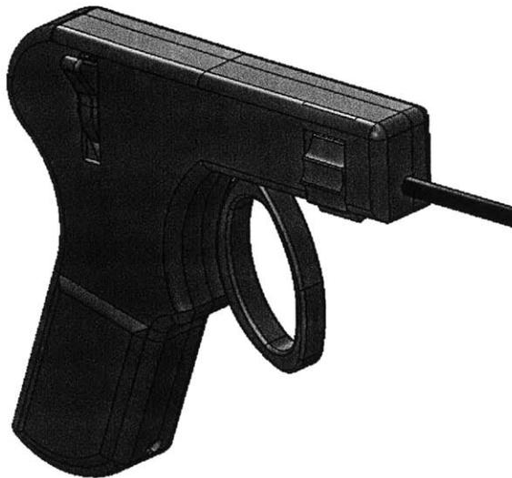
**Figure 8: Thicker pistol grip handle concept.**
