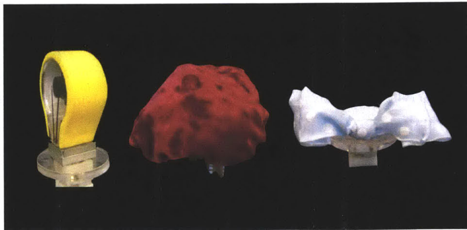
Figure 4-5: Three sensors disguised as a light bulb (color sensor), beret (sound sensor), and bow (tilt sensor).
