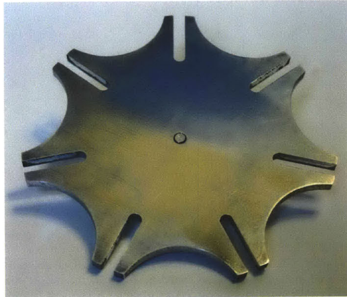
Figure 5-10. The intermittent Geneva wheel produced for this model. This part was cut using a waterjet machine out of aluminum, and then the center axle hole was reamed to size.
