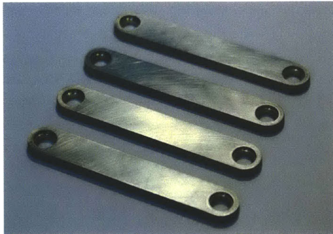
Figure 3-5. Four identical links fabricated for the Peaucellier's linkage model. The brass links were cut on a waterjet machine, and then the pivot holes were drilled and counterbored on a milling machine. Note each link is approximately 2.5 inches long.
