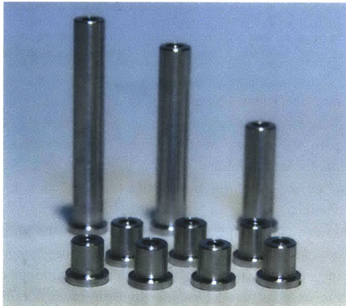
Figure 4-9. All the pivot pins made for the Klann linkage. The pins are made of aluminum, and the longest one is about 1 inch long.
