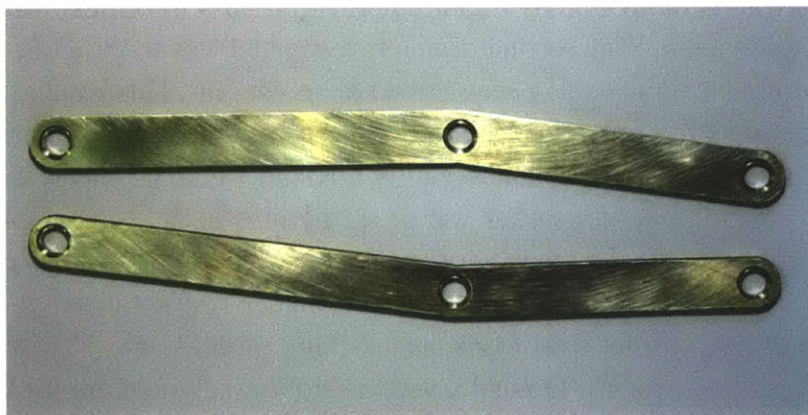
Figure 4-7. Two of the links fabricated for the Klann linkage model. For this particular link, a left and right version was required. The links were made from a brass sheet and are about 5 inches long.
