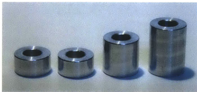
Figure 3-8. Set of spacers fabricated for the Peaucellier's model linkage. The parts are 0.375 inches in diameter and turned on a lathe from aluminum.
