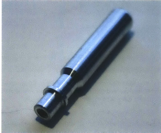
Figure 3-7. Finished handle pin for Peaucellier's linkage, turned from aluminum on a lathe. The features closest in this figure interface with the links and are therefore the same dimensions as a standard pin. The part is approximately 1.5 inches long.
