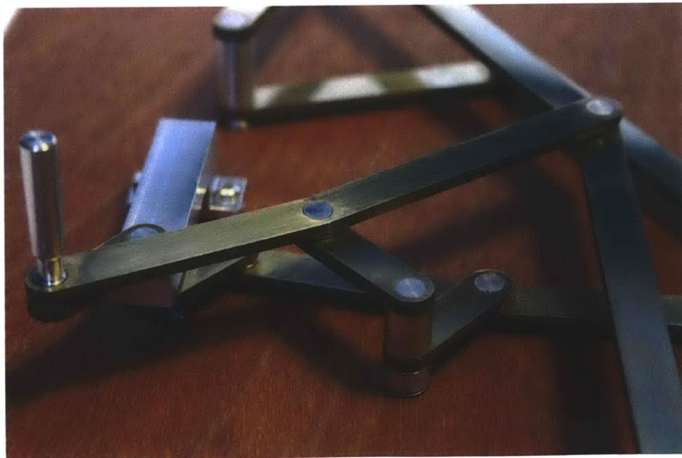
Figure 7-7. Detail of the crank and some of the joints in the Klann linkage model.
