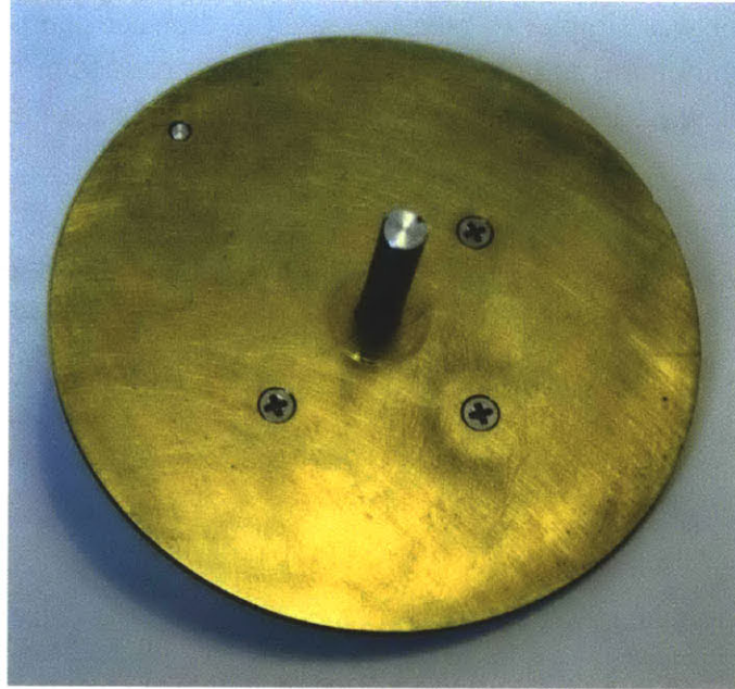
Figure 5-8. Brass input wheel fabricated for the model Geneva drive. The three visible countersunk screws hold the two-piece wheel together.
