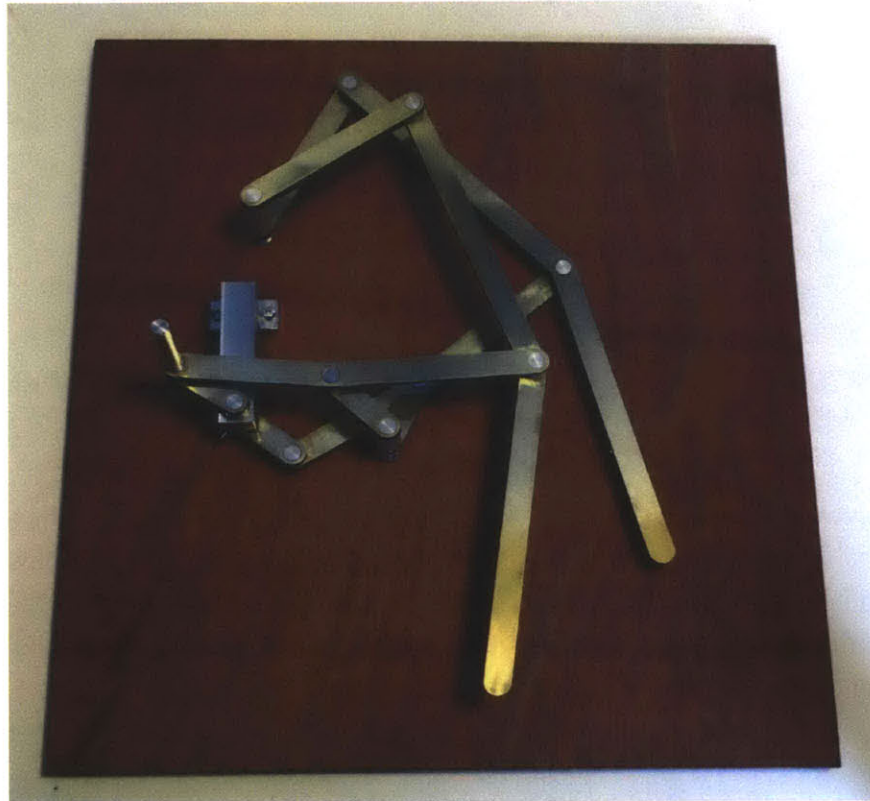
Figure 4-10. The completed Klann's linkage model. The mounting base is oil-treated plywood and is 11 x 12 inches.
