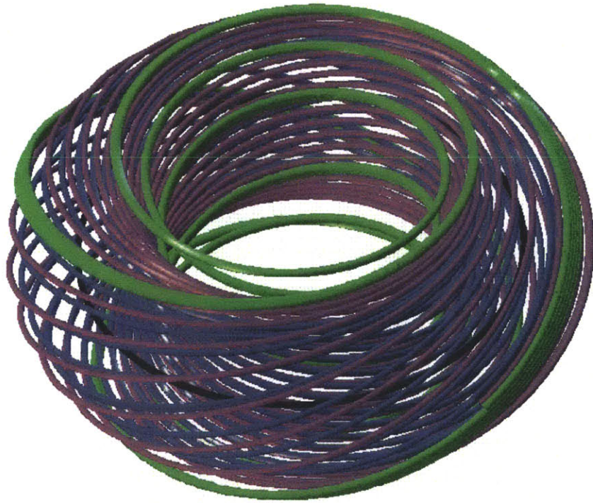
Figure 1-1: Magnetic field lines in a tokamak (toroidal plus poloidal field). Figure courtesy ORNL.
