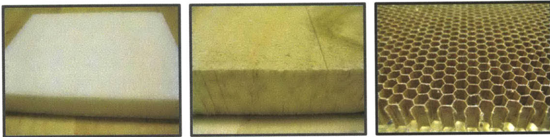
Figure 1-2: Existing core materials: foam, balsa wood, and honeycomb
