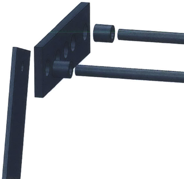
Figure A4: Exploded View of Right Top Link. The threaded rods on the right connect the top links together so that they will move in unison. Bearings were put at each pivot to enable the link to move with less friction. The front wheel axle bar, shown on the far left, was attached to the threaded rod and held in place with a nut (not shown). The threaded rod is wholly unnecessary when the system is made in Guwahati.
