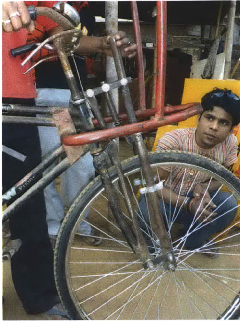
Figure 4: The Alpha-prototype. (a) This photo was taken shortly after the alpha-prototype was assembled and attached to a rickshaw at The Rickshaw Bank factory. Because the left vertical support was made from a straightened bike fork, it had to be further supported by making it into a triangular truss. (b) This is a simplified diagram of the alpha-prototype. Every circle in the diagram is a pivot point. The details of the spring and mount are shown in Figure 5.
