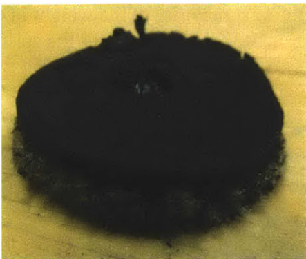
Figure 8: Tire Rubber Donut. The top of the tire rubber donut shown in the photo is the outside of the sidewall of the tire. The fibers near the bottom are the threads that compose the ply.
