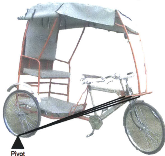
Figure C1: Rickshaw With Ground-based Pivot. The Rickshaw Bank's rickshaw illustrates the distance between the pivot point and the location of the three points of interest on the beta-prototype.
