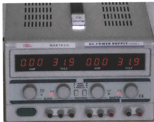
Figure 5: Mastech DC Power Supply HY3005D-3.
