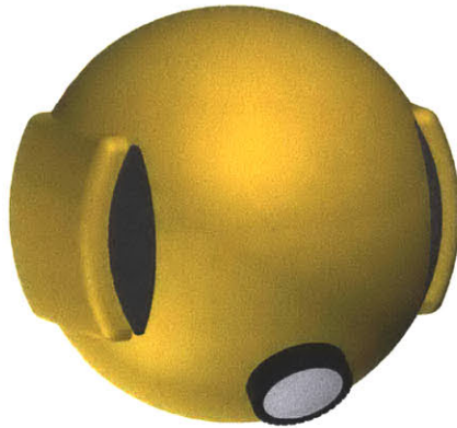
Figure 1-1: This spherical robot has a internal gimbal mechanisms that allows the camera to be rotated freely without the use of external thrusters or propellers. Because of this movement the robot is called The Eyeball.
