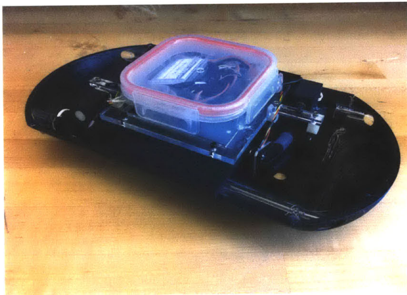
Figure 7-2: Robot made to test the Coanda jet devices. The electronics necessary for the radio control, pumps, and solenoid are held within the opaque box. Tubes direct the water from the Coanda device inside of the boat hull to the outer edge of the hull. These streams of water are used to propel and steer the boat.
