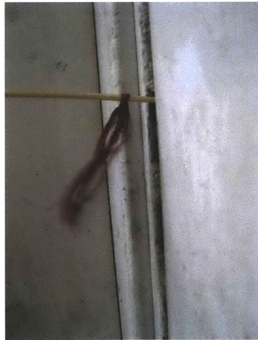
Figure 9: The lowest accessible point of 478 Commonwealth was the basement. The highlighted circle is where the air flow was tested. The direction of the threads shows that air was blowing into the house.
