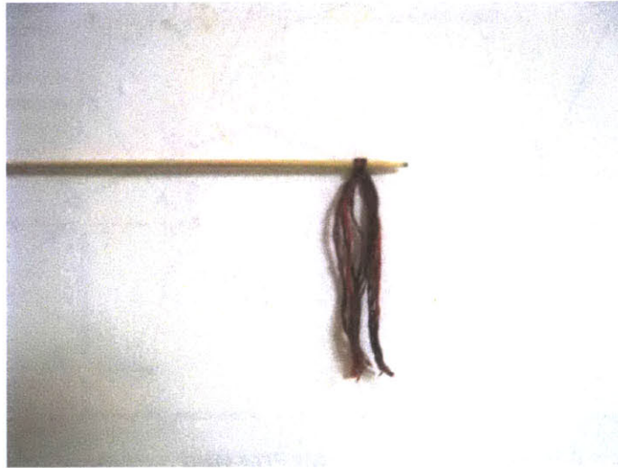
Figure 8: Thread tool constructed to identify air flow direction in 478 Commonwealth
