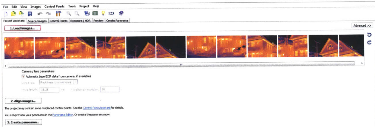
Figure 15: Screenshot of PTGui being used to stitch segmented images into a panorama
